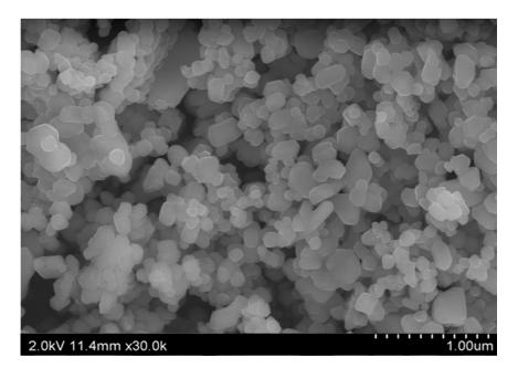
Figure 2. Scanning electronic microscopy (SEM) image of F2.
