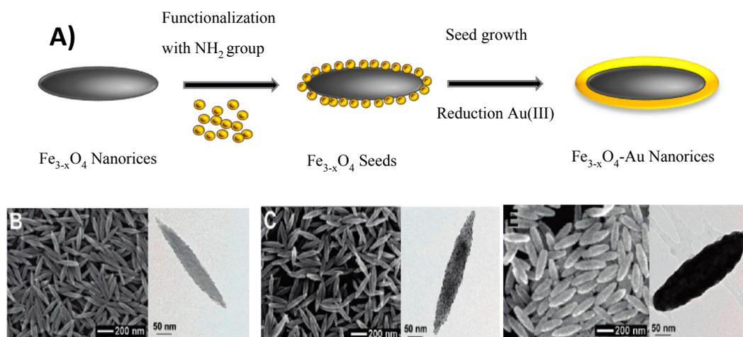
**Figure 8.** (A) Schematic view of the formation of non-spherical core-shell nanoparticles (NPs) starting from anisotropic in shape iron oxide cores. (B–E) Scanning electron microscopy (SEM) (left) and TEM (right) images of (B) hematite cores; (C) core-satellite particles used as seeds; (E) core-shell nanorice particles. Reproduced with permission from [60]. American Chemical Society, 2006.
