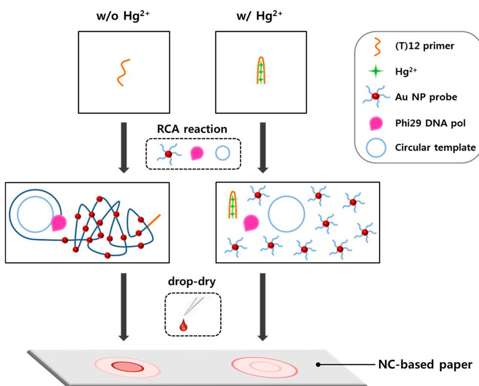
**Figure 1.** Schematic illustration of radial flow assay for  $\text{Hg}^{2+}$  detection.
