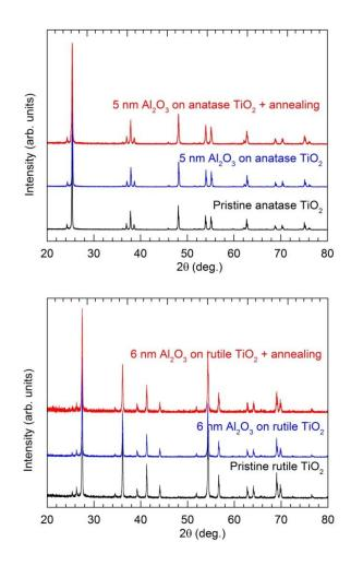
**Figure S1.** XRD patterns of uncoated  $\text{TiO}_2$  and  $\text{Al}_2\text{O}_3$ -coated  $\text{TiO}_2$ , with or without annealing at 500 °C for 12 hours: anatase (top) and rutile (bottom). No signature of  $\text{Al}_2\text{O}_3$  crystal phase was observed, suggesting the amorphous state of the coating layers. The coating has no effects on the crystalline structure of the TiO<sub>2</sub>, even after the annealing.
