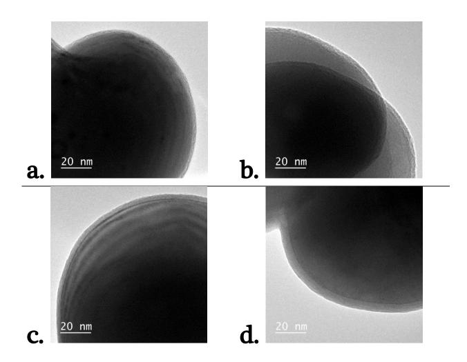
**Figure S4.** TEM micrographs of rutile  $TiO_2$  coated with  $Al_2O_3$  films deposited for (a) 3 cycles, (b) 5 cycles, (c) 10 cycles and (d) 17 cycles. The results demonstrate the growth of uniform  $Al_2O_3$  films. A GPC of 0.34 nm was obtained for the deposition on rutile  $TiO_2$  under the experimental conditions applied for the deposition on anatase  $TiO_2$ .
