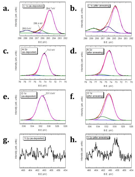
**Figure S3.** XPS spectra of C 1*s*, Al 2*p*, O 1*s* and Ti 2*p* core-levels of anatase TiO<sub>2</sub> coated with 5 nm Al<sub>2</sub>O<sub>3</sub>: as-deposited (a, c. e & g) and after annealing at 500 °C for 12 hours in air (b, d, f & h). No significant changes were observed for the spectra of C 1*s* and Al 2*p* after annealing.
