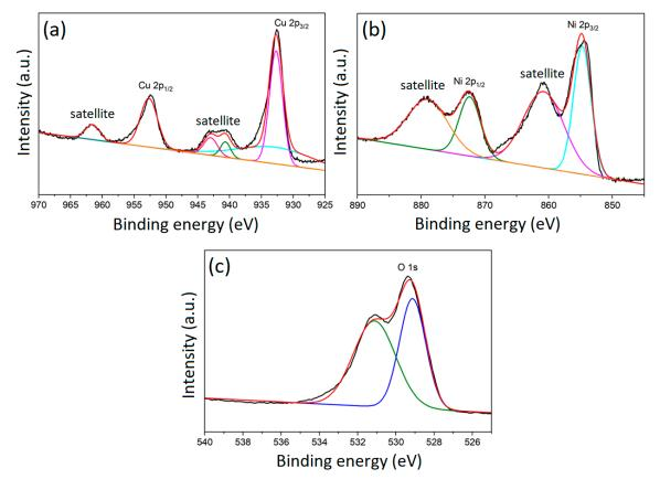
Figure S5. High-resolution XPS spectra for (a) Cu 2p, (b) Ni 2p and (c) O 1s of Cu-Ni\_0.20\_300.
