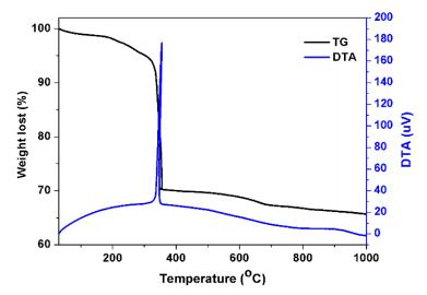
Figure S3. TG-DTA data of Cu-Ni\_0.2. The measurement was carried out in air.
