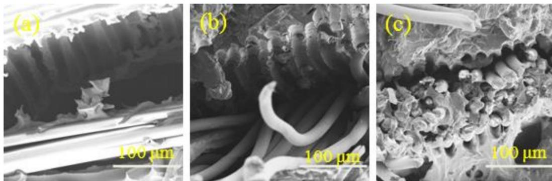
**Figure 12.** Cross section of (a) PF fabric/PVC, (b) PF-1 fabric/PVC, and (c) PF-2 fabric/PVC composites.
