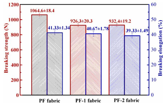
Figure 10. Tensile properties of PET fabrics.
