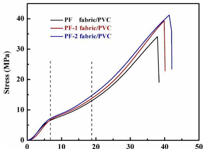
Figure 13. Typical stress–strain curves of the composites.
