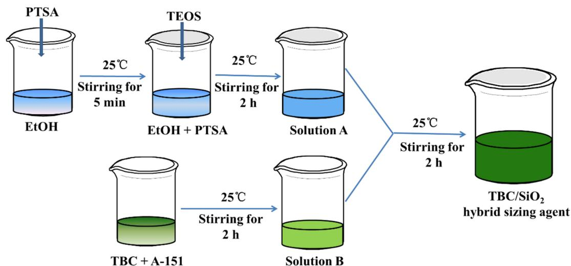
Figure 2. Illustration of the preparation of SiO<sub>2</sub>/TBC hybrid sizing agent.
