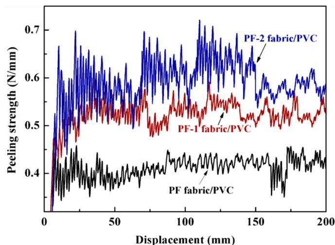
Figure 11. Typical peeling curves of PET fabric/PVC composites.
