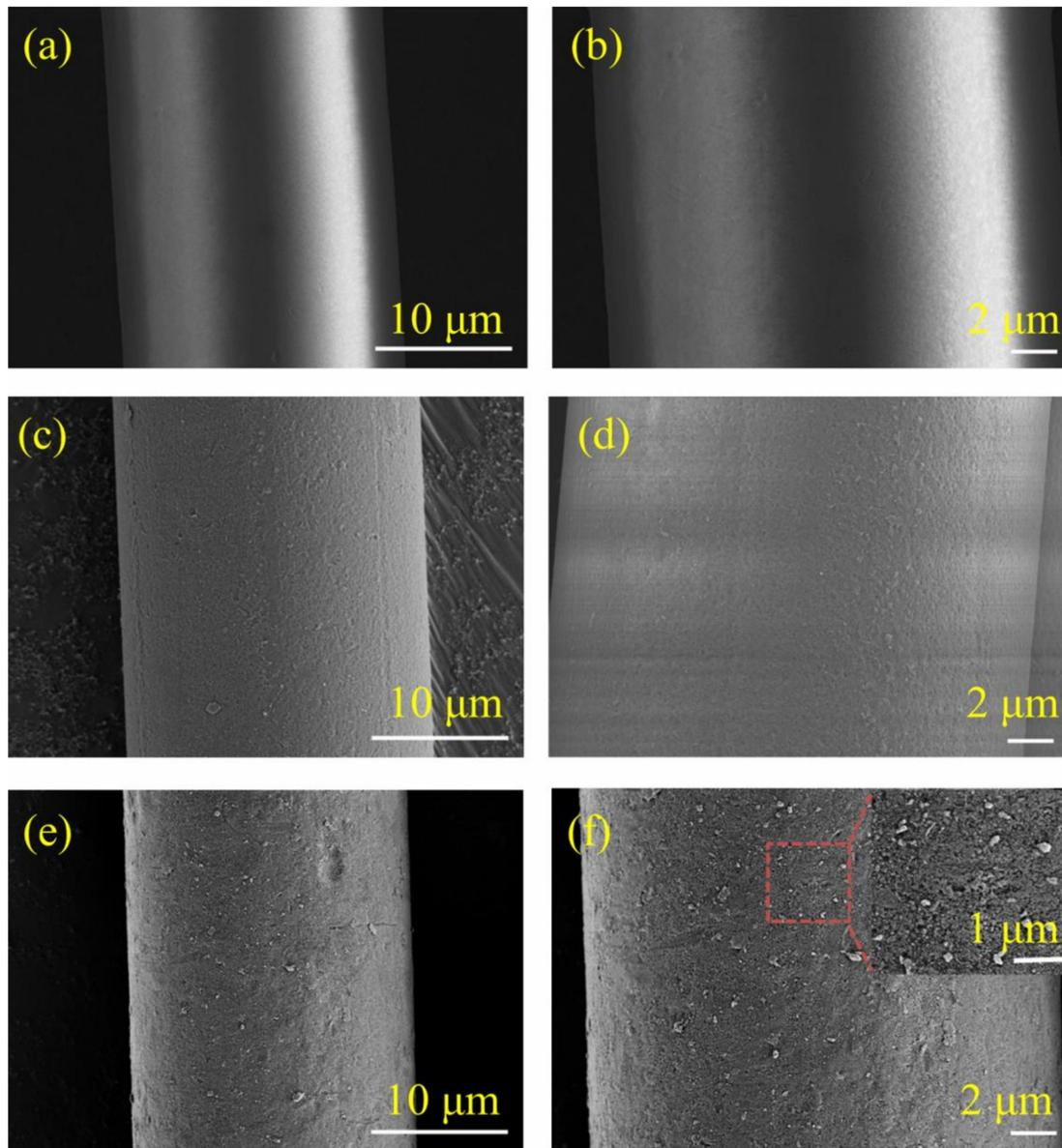
**Figure 6.** SEM images of PET filaments: (a) and (b) PF, (c) and (d) PF-1, (e) and (f) PF-2.
