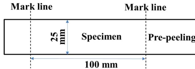
Figure 4. Specimen for peeling strength.
