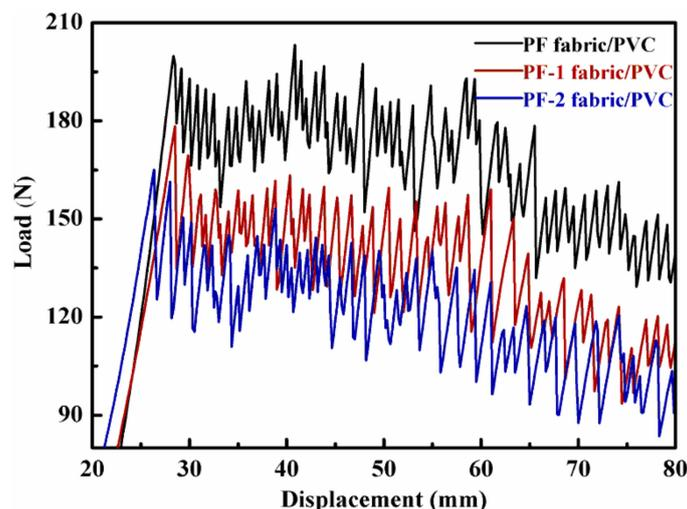
Figure 15. Typical tearing curves of PET fabric/PVC composites.
