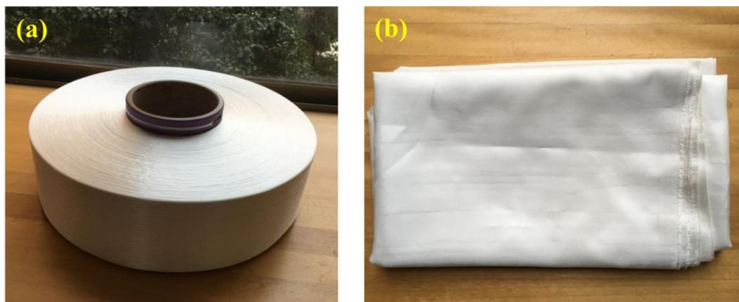
**Figure 1.** Images of PET filament tows and fabrics used in this work: (a) PET filament tows; (b) PET filament fabrics.
