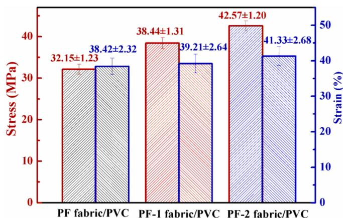
Figure 14. Tensile properties of PET fabric/PVC composites.
