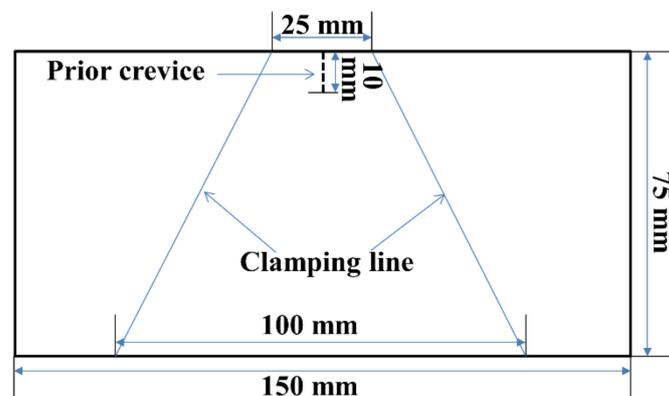
Figure 5. Specimen for tearing strength by trapezoid procedure.
