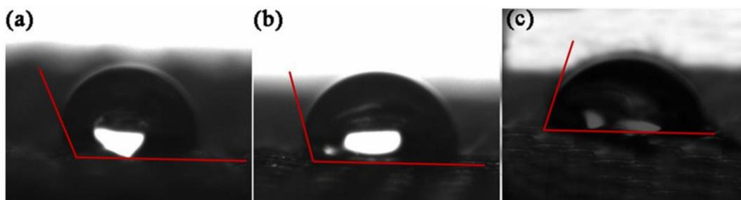
Figure 9. Images of contact angle between TBC and (a) PF fabric, (b) PF-1 fabric, and (c) PF-2 fabric.
