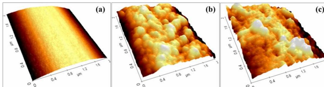
**Figure 7.** AFM images of PET filaments: (a) PF, (b) PF-1, (c) PF-2.
