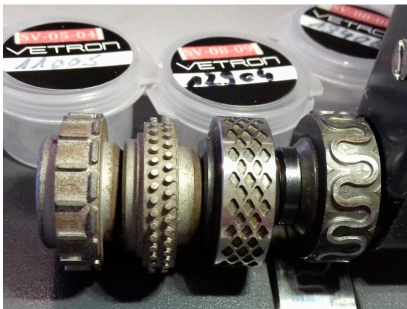
**Figure 1.** Anvil wheels chosen for this study. From left to right: T-stitch, point 2-rowed, diamond, and omega.
