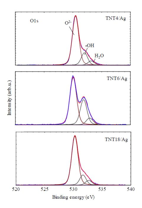
**Figure S2. The d**econvolution of O(1s) peak in the XPS spectrum of TNT/Ag coatings.
