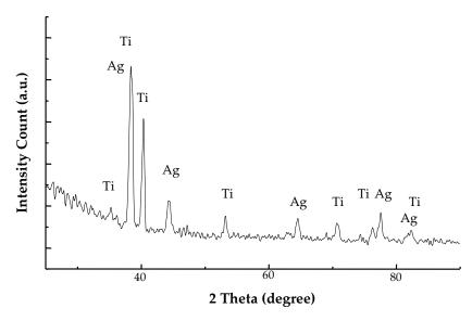
**Figure S1.** X-ray diffraction pattern of silver grains deposited on the surface of TNT6; Ag: 38.1 (111), 44.6 (200), 64.7 (220), 77.5 (311) and 81.5 (222), Ti: 35.1 (100), 38.4 (002), 40.2 (101), 53.0 (102), 70.7 (103), 76.3 (112) and 82.3 (004) (results of these investigations indicate on the amorphousness of the TNT6 coating, CVD,  $T_D = 553$  K, p = 3 mbar, t = 30 min., m = 10 mg).
