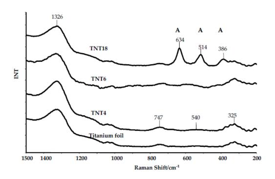
**Figure S3.** Raman specta of TNT samples heated up to 573 K.
