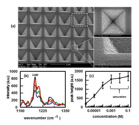
**Figure 11.** (a) Electron micrographs of the pyramidal wells in Klarite showing the roughened gold structure. Reproduced with permission from the Royal Society of Chemistry, 2010 [121]; (b) SERS spectra of ibuprofen as a function of concentration and (c) Plot of 1180 cm<sup>-1</sup> peak height as a function of ibuprofen concentration. Reproduced with permission from Samedan Ltd, 2010 [122].
