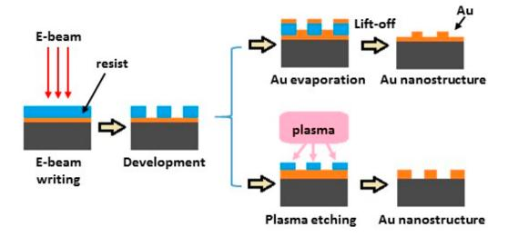
Figure 10. Schematic of the two fabrication processes used to prepare nanostructured SERS substrates.
