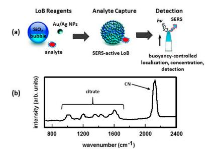
**Figure 15.** (a) The basic components of a lab-on-a-bubble (LoB) assay for SERS-based detection of an analyte; (b) SERS spectra of cyanide and citrate on LoB. Reproduced with permission from the American Chemical Society, 2012 [158].
