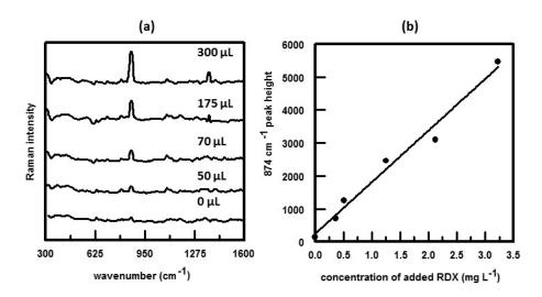
**Figure 5.** (a) SERS spectra of contaminated groundwater sample obtained using the standard addition method. Volume of RDX stock solution (177.7 mg  $L^{-1}$ ) added to each sample is indicated. Spectra were obtained using 785 nm excitation; (b) Standard addition curve for determining the RDX concentration in the groundwater sample. Reproduced with permission from John Wiley and Sons, 2010 [39].
