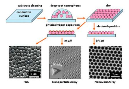
**Figure 8.** Schematic representation of the nanosphere lithography process for fabricating metal film over nanosphere (FON), periodic nanoparticle arrays, or nanovoid arrays. Reproduced with permission from Royal Society of Chemistry, 2008 [95].
