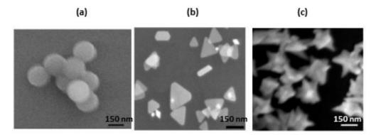
**Figure 1.** SEM images of the following gold nanostructures: (**a**) nanospheres; (**b**) nanotriangles, and (**c**) nanostars. Reproduced with permission from Royal Society of Chemistry, 2014 [59].
