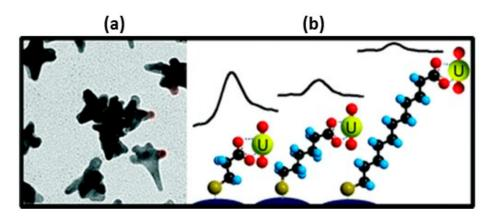
**Figure 14.** (a) SEM of carboxylic acid terminated alkanethiol derivatized Au nanostars; (b) Schematic of the SAM-uranyl interaction and the resultant Raman peaks due to uranyl. Reproduced with permission from the Royal Society of Chemistry, 2016 [139].
