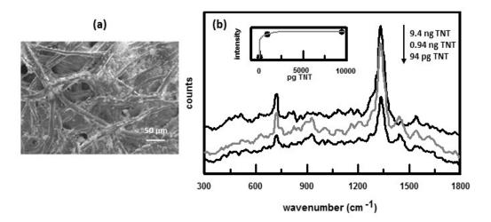
**Figure 7.** (a) SEM of printed Au NPs on filter paper; (b) SERS spectra of TNT. Concentrations are indicated. Inset shows the variation of SERS intensity of  $NO_2$  band as a function of concentration. Reproduced with permission from Hindawi Publishing Corporation, 2012 [42].
