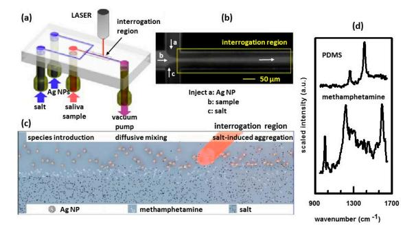
**Figure 3.** (a) Schematic of the flow-focusing microfluidic device used for controlled Ag-NP aggregation; (b) Microphotograph of the flow-focusing junction; (c) Schematic of the reactions occurring between the analyte, Ag NPs, and salt ions; (d) Raman spectrum of PDMS that comprises the channel is shown as well as the SERS spectrum of methamphetamine in the channel. Reproduced with permission from American Chemical Society, 2013 [65].
