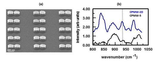
**Figure 13.** (a) SERS image of a section of a representative elevated Au ellipse dimer array. Array has been tilted at 30° such that the underlying nanopads are visible; (b) SERS spectra of two groundwater samples collected from a contaminated US DoD Navy site. The cationic thiol DMAH<sup>+</sup> has been chemisorbed on the dimers Vertical dashed line indicates the perchlorate peak. Reproduced with permission from John Wiley and Sons, 2017 [22].
