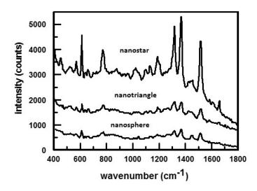
**Figure 2.** Comparison of 5  $\mu$ M rhodamine 6G SERS spectra in suspensions of gold nanostars, nanotriangles, and aggregated nanospheres. The SERS response was negligible for unaggregated nanosperes. SEM images of the nanostructures are shown in Figure 1. Spectra were obtained using a laser excitation of 785 nm. Reproduced with permission from Royal Society of Chemistry, 2014 [59].
