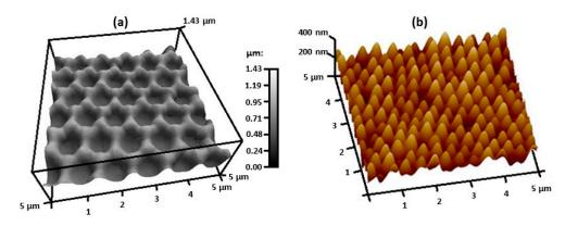
**Figure 9.** AFM images obtained for flexible SERS substrates obtained by (**a**) method that combines soft lithography with nanosphere lithography, 2013 [98] and (**b**) R2R UV-NIL, 2017 [99]. Reproduced with permission from Nature Publishing Group.
