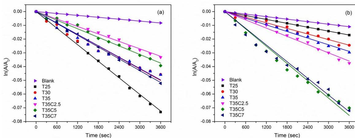
**Figure 7.** Kinetics plot of selected thin films of methylene blue degradation under (a) UV and (b) visible light irradiation.
