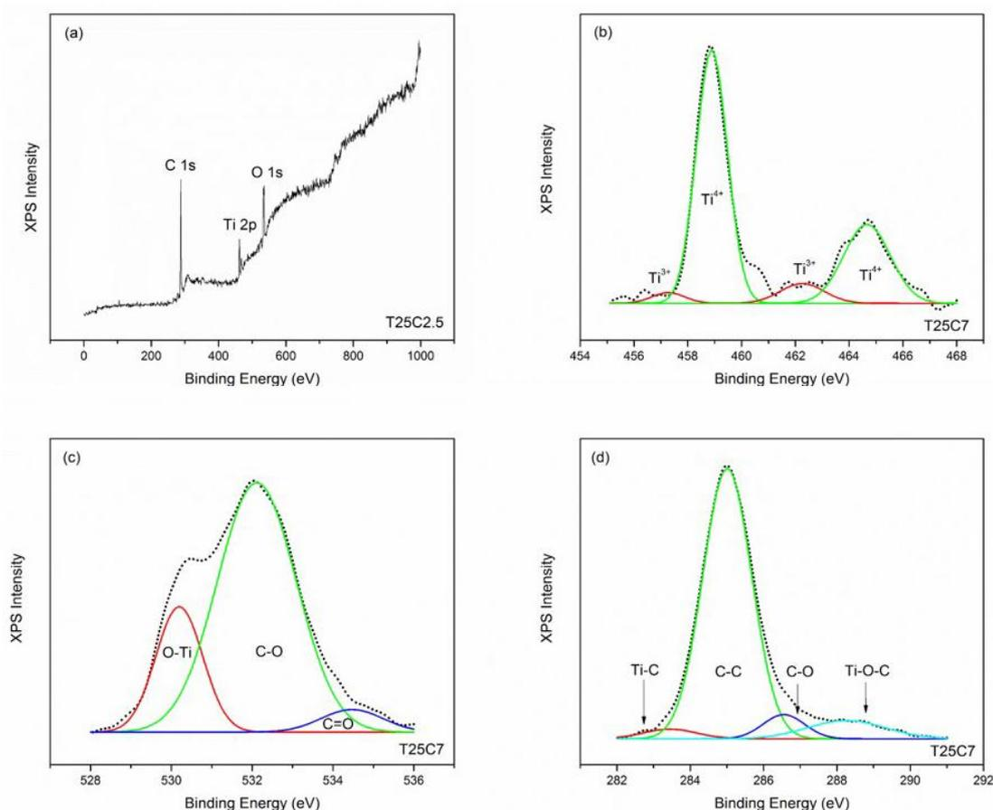
**Figure 5.** X-ray photoelectron spectroscopy (XPS) results of selected C-doped samples: (a) Survey spectrum (sample T25C2.5); (b) Ti 2p spectrum (sample T25C7); (c) O 1s spectrum (sample T25C7); (d) C 1s spectrum (sample T25C7).
