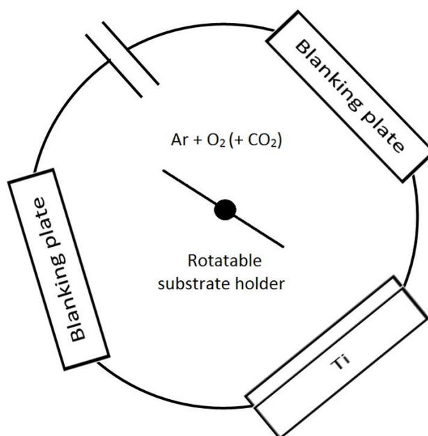
**Figure 1.** Schematic representation of the Teer UDP350 sputtering rig.
