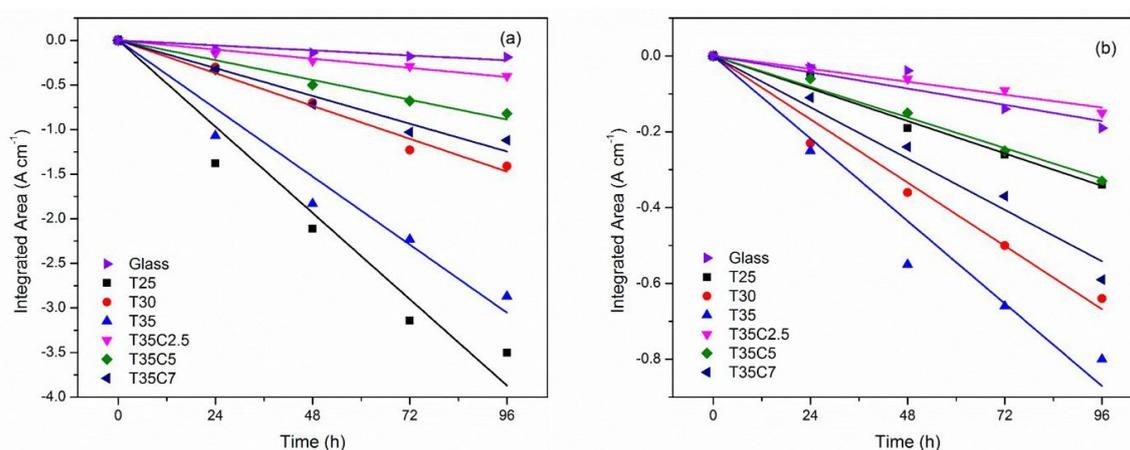
**Figure 8.** Plots of the integrated area changes of the FTIR spectra of the stearic acid peaks ( $3000\text{--}2700\text{ cm}^{-1}$ ) for selected C-doped and undoped  $\text{TiO}_2$  samples under: (a) UV light irradiation; (b) visible light irradiation.
