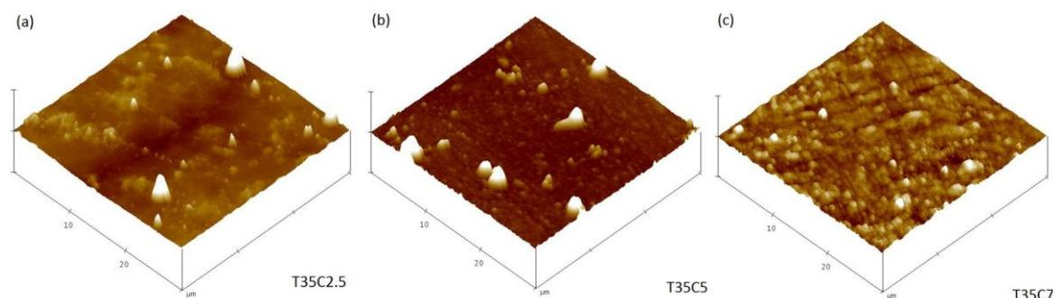
**Figure 3.** AFM images of selected C-doped coatings deposited on glass substrate (a) T35C2.5; (b) T35C5; (c) T35C7.
