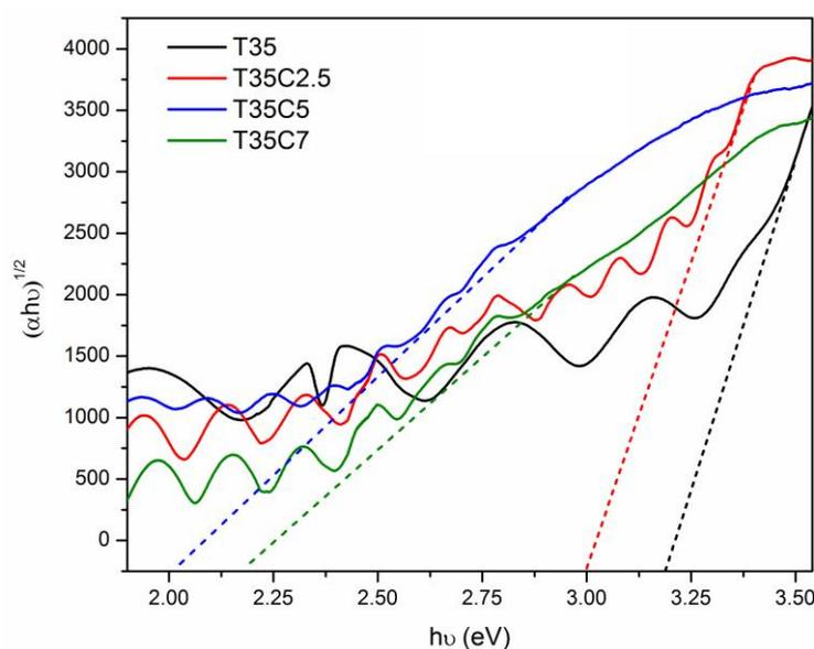
**Figure 6.** Examples of band gap calculations for selected C-doped and undoped titania samples (deposited at 35% OEM setpoint).
