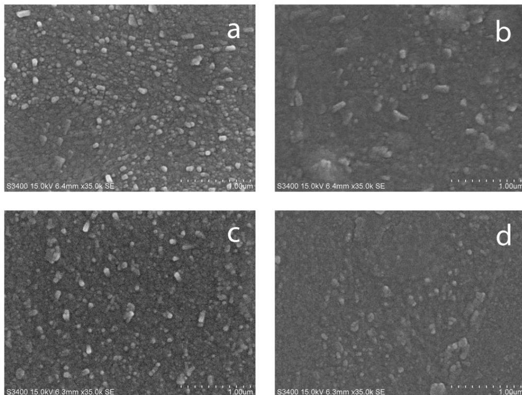
**Figure 2.** Scanning electron microscopy (SEM) images of selected titania and C-doped titania coatings deposited on glass substrate (a) T35; (b) T35C2.5; (c) T35C5; (d) T35C7.
