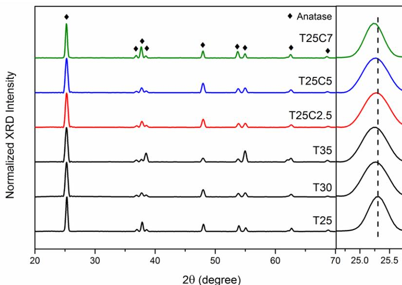
**Figure 4.** X-ray diffraction (XRD) patterns of selected C-doped and undoped TiO<sub>2</sub> coatings (25% optical emission monitoring (OEM) setpoint) deposited on glass substrates and annealed at 873 K.
