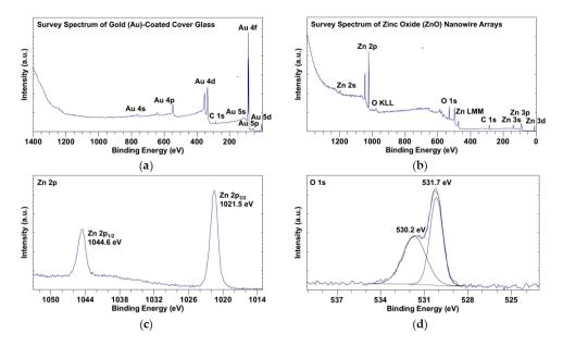
**Figure 2.** X-ray photoelectron spectroscopy (XPS) spectra of Au-coated cover glass and ZnO nanowire arrays: (**a**) survey spectrum of Au-coated cover glass; (**b**) survey spectrum of ZnO nanowire arrays; (**c**) Zn 2p spectrum of ZnO nanowire arrays; (**d**) deconvoluted O 1s spectrum of ZnO nanowire arrays.
