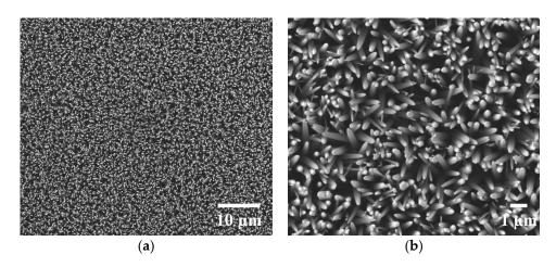
**Figure 1.** Scanning electron microscopy (SEM) images of zinc oxide (ZnO) nanowire arrays: (**a**) SEM image at a magnification of  $2500 \times$ ; (**b**) SEM image at a magnification of  $10,000 \times$ .
