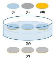
Figure 6. Schematic of synthesis of ZnO nanowire arrays using a seedless solution-based method.
