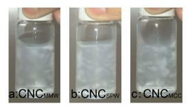
**Figure 4.** Flow birefringence of cellulose nanocrystal suspensions between two cross polarizers (a) CNC<sub>MMW</sub>, (b) CNC<sub>SPW</sub>, and (c) CNC<sub>MCC</sub>.
