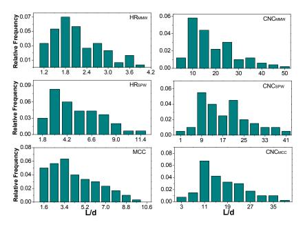
Figure 3. Aspect ratio distributions of HR<sub>MMW</sub>, HR<sub>SPW</sub>, MCC, and their CNCs.
