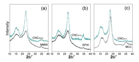
**Figure 5.** X-ray powder diffractograms of the hydrolyzed residuals (HRs), MCC, and the CNCs. (a) MMW and its resulted  $CNC_{MMW}$ ; (b) SPW and its resulted  $CNC_{SPW}$ ; (c) MCC and its resulted  $CNC_{MCC}$ .
