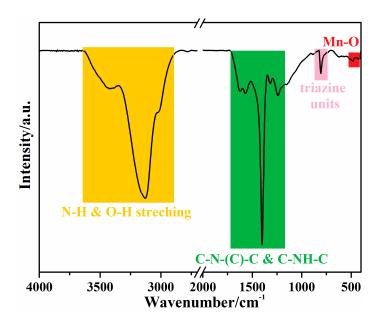
Figure S2. FT-IR spectrum of the g-C<sub>3</sub>N<sub>4</sub>/rGO/MnO<sub>2</sub> Ternary Nanocomposite.
