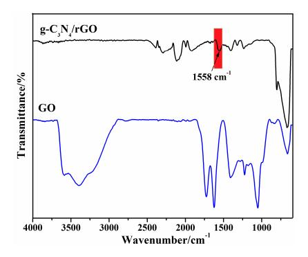
Figure S1 FT-IR curves of the g-C<sub>3</sub>N<sub>4</sub>/rGO nanocomposite
