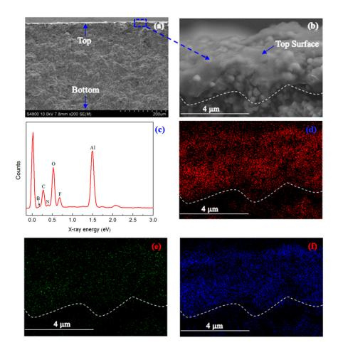
**Figure 2.** (a) SEM image, (b) Partially magnified SEM image, (c) Total element mapping, (d) Element C mapping, (e) Element B mapping and (f) Element F mapping of [emim][BF<sub>4</sub>] confined in mesoporous polymer membrane on Al<sub>2</sub>O<sub>3</sub> support.
