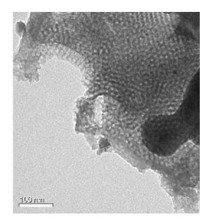
**Figure 3.** Transmission electron micro (TEM) image of mesoporous phenolic resin scratched from Al<sub>2</sub>O<sub>3</sub> support.
