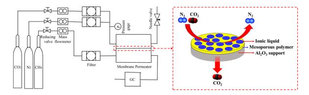
Figure 8. Schematic diagram of membrane permeation unit (GC: gas chromatograph, P: Pressure).
