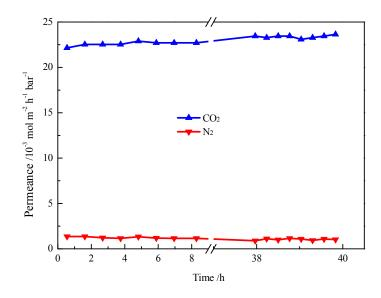
**Figure 7.** CO<sub>2</sub> and N<sub>2</sub> separation stability of [emim][BF<sub>4</sub>] confined in mesoporous polymer membrane on Al<sub>2</sub>O<sub>3</sub> support,  $\Delta P = 1.5$  bar, feed concentration CO<sub>2</sub>/N<sub>2</sub> = 50/50% (v/v).
