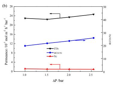
**Figure 5.** Effect of trans-membrane pressure difference ( $\Delta P$ ) on permeances and selectivities of [emim][BF<sub>4</sub>] confined in mesoporous polymer membrane on Al<sub>2</sub>O<sub>3</sub> support at 25 °C. (**a**) CO<sub>2</sub>/N<sub>2</sub> ideal selectivity; (**b**) CO<sub>2</sub>/N<sub>2</sub> actual selectivity, feed concentration CO<sub>2</sub>/N<sub>2</sub> = 50/50% (v/v).
