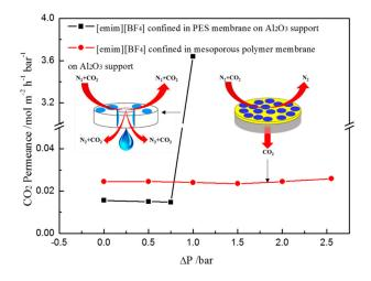
**Figure 6.** Stability comparison between [emim][BF<sub>4</sub>] confined in mesoporous polymer membrane on Al<sub>2</sub>O<sub>3</sub> support and [emim][BF<sub>4</sub>] confined in polyethersulphone (PES) macroporous membrane on Al<sub>2</sub>O<sub>3</sub> support.
