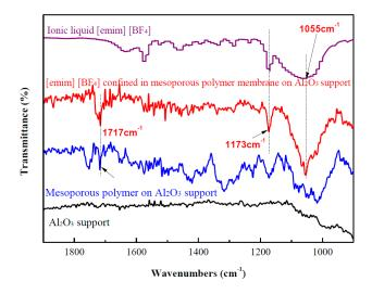
**Figure 1.** Fourier-transform infrared (FTIR) spectra of Al<sub>2</sub>O<sub>3</sub>, mesoporous polymer membrane on Al<sub>2</sub>O<sub>3</sub> support, [emim][BF<sub>4</sub>] confined in mesoporous polymer membrane on Al<sub>2</sub>O<sub>3</sub> support, and pure [emim][BF<sub>4</sub>].
