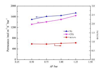
**Figure 4.** Effect of trans-membrane pressure difference ( $\Delta P$ ) on permeances and CO<sub>2</sub>/N<sub>2</sub> ideal selectivities of mesoporous polymer membrane on Al<sub>2</sub>O<sub>3</sub> support.
