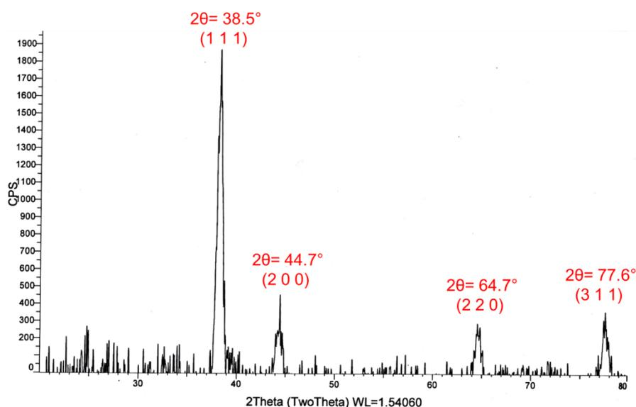
**Figure 5.** X-ray diffraction (XRD) pattern of sample 1 (S1), showing the face centered cubic (FCC) crystalline metallic silver nanoparticles (AgNPs). The intensity in vertical axis is measured in counts per second (CPS) and diffraction angle (2 theta) measured is taken along horizontal axis. The value of wavelength (WL in angstrom) is also mentioned in the figure.
