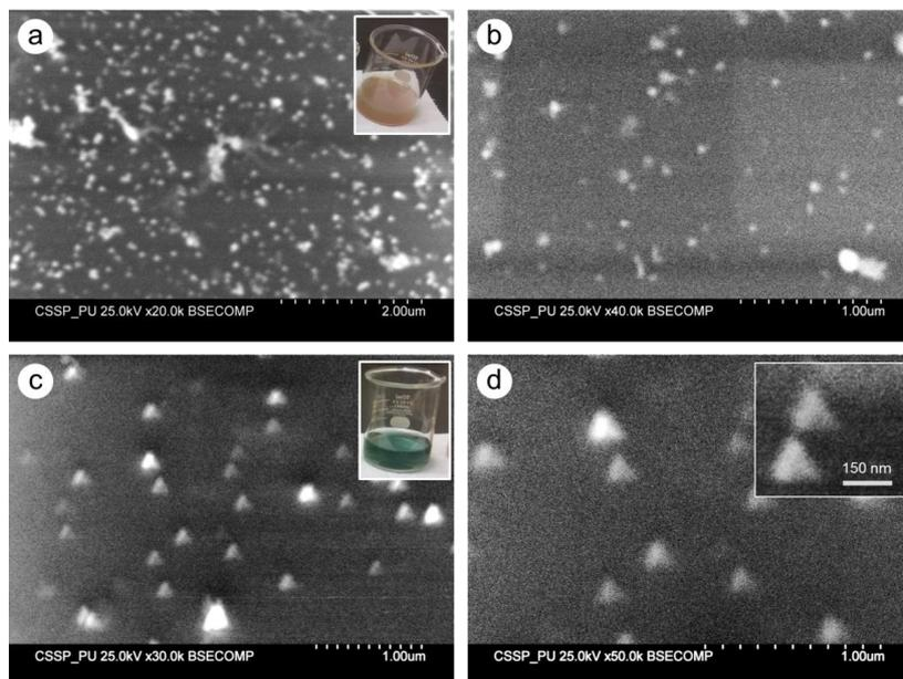
**Figure 3.** SEM images of Sample 1 at lower (a) and higher (b) magnification showing the spherical morphology of the particles. The triangle-shaped silver particles are represented in (c) and (d) at different magnifications. The inset showed the color of sample S1 and sample S2 solution the beaker.
