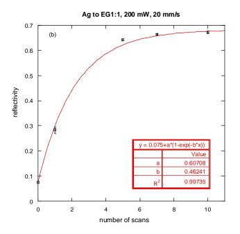
**Figure 7.** (a) Thickness of the silver film (b) reflectivity for 532 nm wavelength light *versus* number of laser scans (symbols: experimental data, lines: fitted curves).
