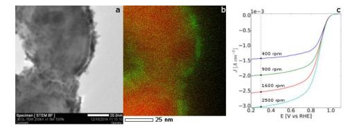
**Figure 11.** STEM image of platinum on nickel nanofibres after the galvanic displacement (**a**), overlay of the EDX maps of Ni (**red**) and Pt (**green**) (**b**) and oxygen reduction reaction (ORR) at 5 mV/s in 0.1 M HClO<sub>4</sub> saturated with O<sub>2</sub> at 400, 900, 1600, 2500 RPM (**c**).
