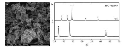
**Figure 9.** SEM micrograph of a sponge-like Ni<sub>3</sub>N structure (obtained from NiO nanofibers derived from PVP and nickel acetate in DMF/ethanol) (**a**) and the corresponding XRD diffractogram (**b**) before and after the two-step complete conversion in NH<sub>3</sub>. JCPDS reference: Ni<sub>3</sub>N 00-010-280, Ni 96-151-2527.
