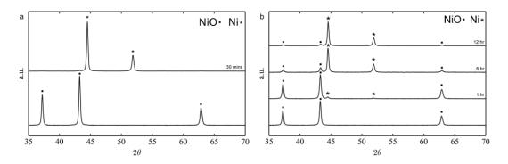
**Figure 5.** X-ray diffraction (XRD) diffractograms of the conversion of NiO to Ni fibers at 250 °C in pure hydrogen (**a**) vs.  $H_2/Ar$ ; and (**b**) Joint Committee on Powder Diffraction Standards (JCPDS) reference: NiO 96-101-0094, Ni 96-151-2527.
