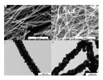
**Figure 6.** SEM micrographs of NiO ribbons (obtained from polyvinylpyrrolidone (PVP) and nickel acetate in ethanol) and transmission electron microscope (TEM) micrographs of NiO nanofibers (obtained from PVP and nickel acetate in DMF/ethanol) before (**a**,**c**) and after reduction at 250 °C in H<sub>2</sub> (**b**,**d**).
