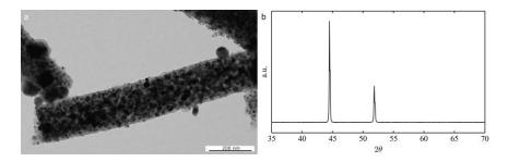
**Figure 8.** TEM micrograph of Ni/C composite fibers (obtained from PVP and nickel acetate in DMF/ethanol at 700 °C under nitrogen (**a**) and the corresponding XRD diffractogram (**b**) JCPDS reference: Ni 96-151-2527.
