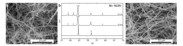
**Figure 10.** SEM of Ni fibers before (**a**) and after thermal treatment under  $NH_3$  (**c**) and XRD diffractogram of fibers with different degrees of conversion to the nitride phase (**b**) JCPDS reference: Ni<sub>3</sub>N 00-010-280, Ni 96-151-2527.
