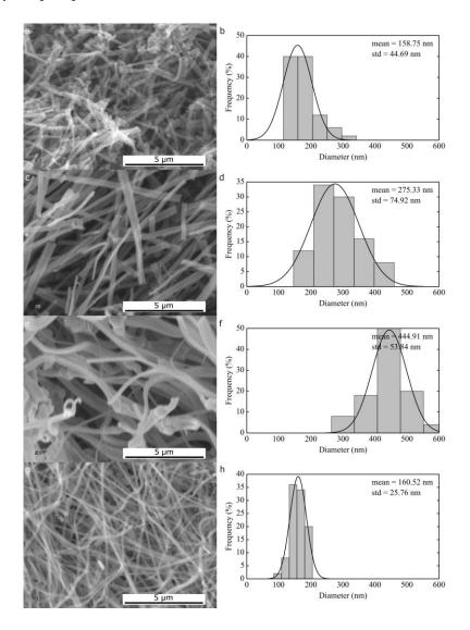
**Figure 3.** SEM micrographs and corresponding histograms of size distribution of NiO electrospun in the same conditions as 9 (**a**,**b**), 10 (**c**,**d**), 11 wt % (**e**,**f**) polyvinylpyrrolidone and nickel acetate in ethanol (**a**,**b**) and in ethanol:dimethylformamide (7:3 vol.) (**g**,**h**).
