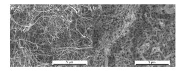
**Figure 7.** SEM micrographs of electrospun Ni (from polyvinylalcohol and nickel acetate in water) obtained after reduction in H<sub>2</sub> at 250 °C (**a**) and 400 °C (**b**).
