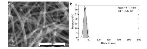
**Figure 2.** (a) Scanning electron microscopy (SEM) micrograph and (b) corresponding histogram of fiber size distribution of NiO fibers obtained from 12 wt % polyvinylalcohol and 12 wt % nickel acetate in H<sub>2</sub>O.
