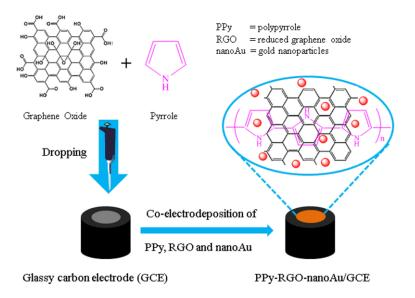
**Figure 1.** Schematic illustration of polypyrrole-reduced graphene oxide-gold nanoparticles biocomposite (PPy–RGO–nanoAu)-modified glassy carbon electrode (GCE).
