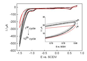
**Figure 2.** Typical cyclic voltammograms (CVs) of pyrrole/graphene oxide/GCE in HAuCl<sub>4</sub> aqueous solution for 10 cycles with a scan rate of 25 mV/s. The scanning potential ranged from -1.5 V to 0.8 V vs. saturated calomel electrode (SCE). The arrows indicate the trend of redox current response during potential cycles.
