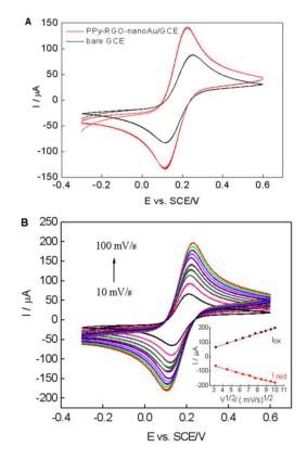
**Figure 4.** (A) CVs of the bare GCE (black line) and PPy-RGO-nanoAu/GCE (red line) in 0.1 M KCl containing 5 mM [Fe(CN)<sub>6</sub>]<sup>3-/4-</sup> (1:1) with a scan rate of 50 mV/s; (B) CVs of the PPy-RGO-nanoAu/GCE recorded at 10, 20, 30, 40, 50, 60, 70, 80, 90 and 100 mV/s in 0.1 M KCl containing 5 mM [Fe(CN)<sub>6</sub>]<sup>3-/4-</sup> (1:1). Inset: linear dependence of anodic and cathodic peak currents ( $I_{ox}$  and  $I_{red}$ ) vs. the square-root of the scan rate.
