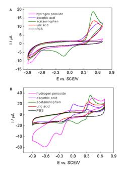
**Figure 6.** CVs of (**A**) bare GCE and (**B**) PPy–RGO–nanoAu/GCE in PBS containing 1 mM uric acid, 1 mM ascorbic acid, 1 mM acetaminophen, and 0.5 mM H<sub>2</sub>O<sub>2</sub>, respectively. Scan rate: 50 mV/s.
