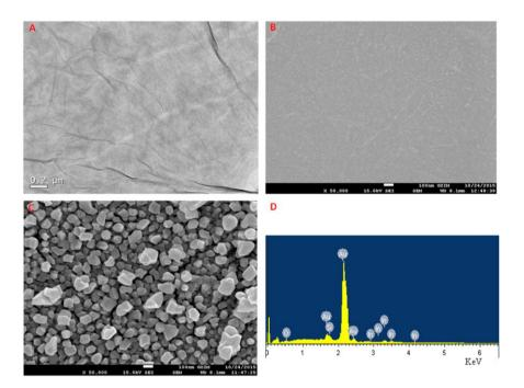
**Figure 3.** (**A**) Typical transmission electron microscopy image of graphene oxide; (**B**) scanning electron microscopy images of pyrrole/graphene oxide; and (**C**) PPy–RGO–nanoAu; and (**D**) energy dispersive spectroscopy spectrum of PPy–RGO–nanoAu.
