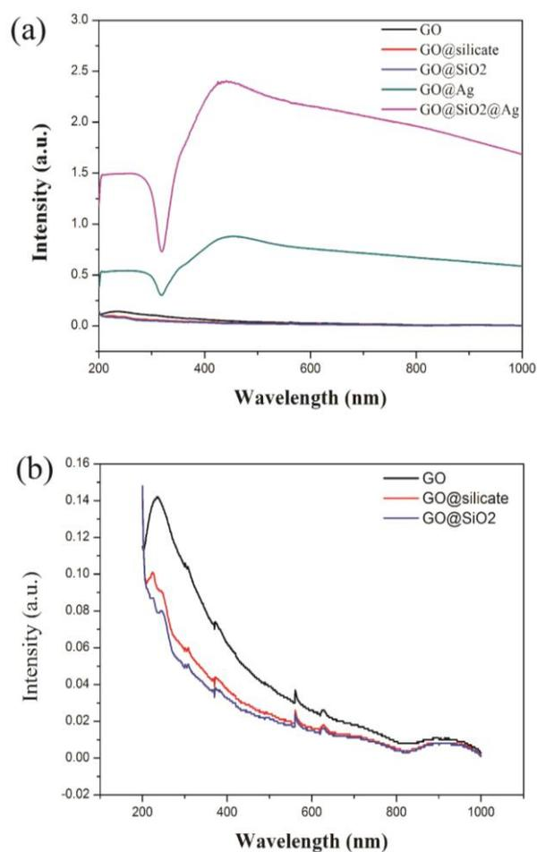
**Figure S3.** UV-vis spectroscopy (a) and enlargement (b) of graphene oxide (GO), silica-coated graphene oxide (GO@silicate), thiolated silica-coated graphene oxide (GO@SiO<sub>2</sub>), silver nanoparticle-embedded silica-coated graphene oxide (GO@SiO<sub>2</sub>@Ag) and silver nanoparticle-embedded graphene oxide (GO@Ag).
