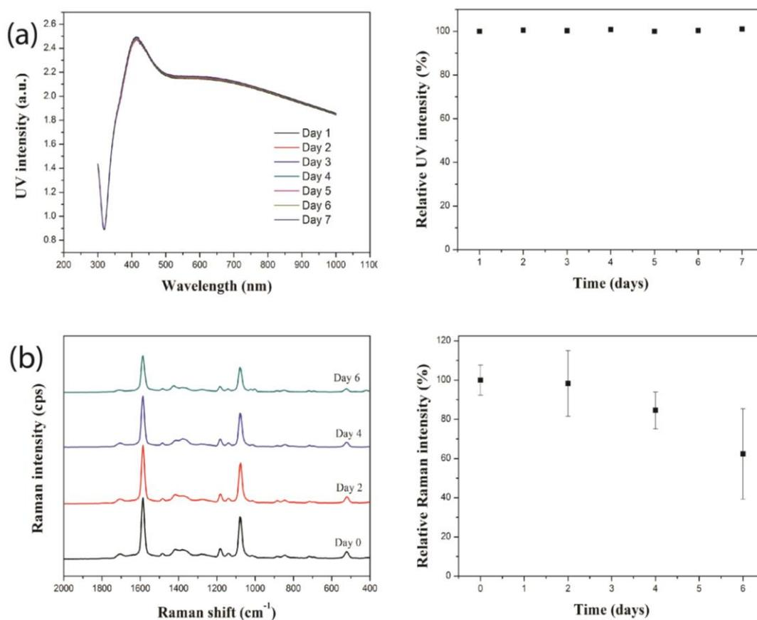
**Figure S7.** (a) UV spectra and (b) SERS spectra of GO@SiO<sub>2</sub>@Ag NPs which stored in ethanol solution at room temperature in darkness. The spectra range from 400–2000 nm. Herein 10  $\mu\text{M}$  4-MBA (1 mL) was incubated with GO@SiO<sub>2</sub>@Ag NPs and measured Raman spectroscopy.
