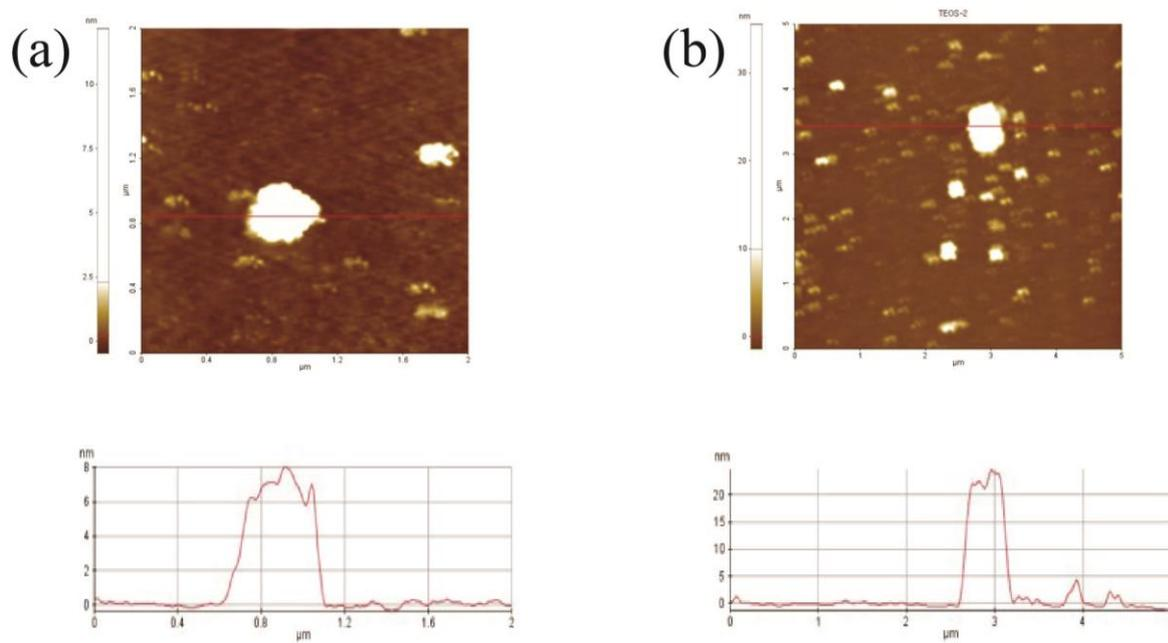
**Figure S1.** Atomic force microscopy images and histogram of (a) graphene oxide and (b) silica-coated GO. GO concentration is 1 mg/mL.
