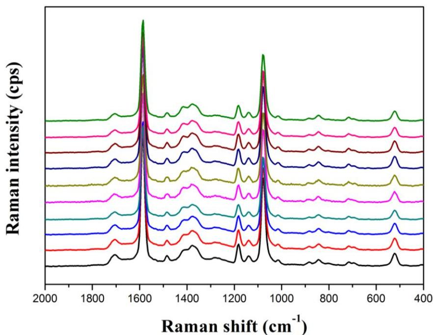
**Figure S6.** SERS spectra of 10  $\mu\text{M}$  4-MBA in ethanol solution contain GO@SiO<sub>2</sub>@Ag NPs (1 mg/mL). The spectra range from 400–2000 nm.
