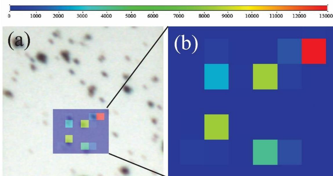
**Figure S5.** (a) Merged image of 2D Raman mapping and optical images of GO@SiO<sub>2</sub>@Ag NPs with 1 mM 4-mercaptobenzoic acid. (b) 2D Raman mapping of GO@SiO<sub>2</sub>@Ag NPs. GO concentration is 1 mg/mL. Laser power is 10 mW, wavelength is 532 nm, integration time is 5 s, and laser spot is 2  $\mu$ m.
