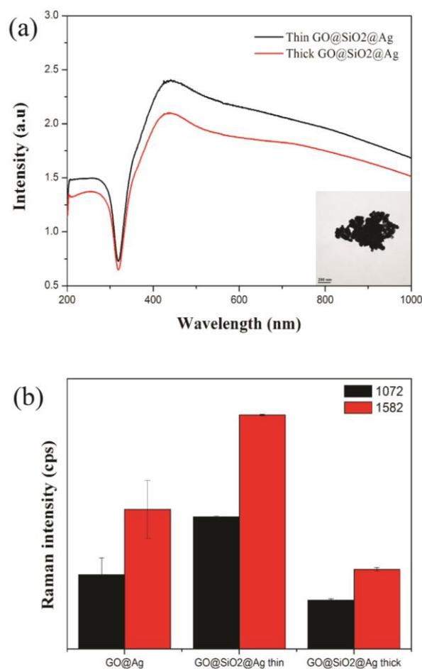
**Figure S4.** (a) UV spectra and (b) SERS intensity of thin and thick GO@SiO<sub>2</sub>@Ag NPs in EtOH solution with 1 mM 4-mercaptobenzoic acid. Inset is TEM image of thick GO@SiO<sub>2</sub>@Ag NPs. GO concentration is 1 mg/mL, laser power is 10 mW, wavelength is 532 nm, integration time is 5 s, and laser spot is 2  $\mu$ m.
