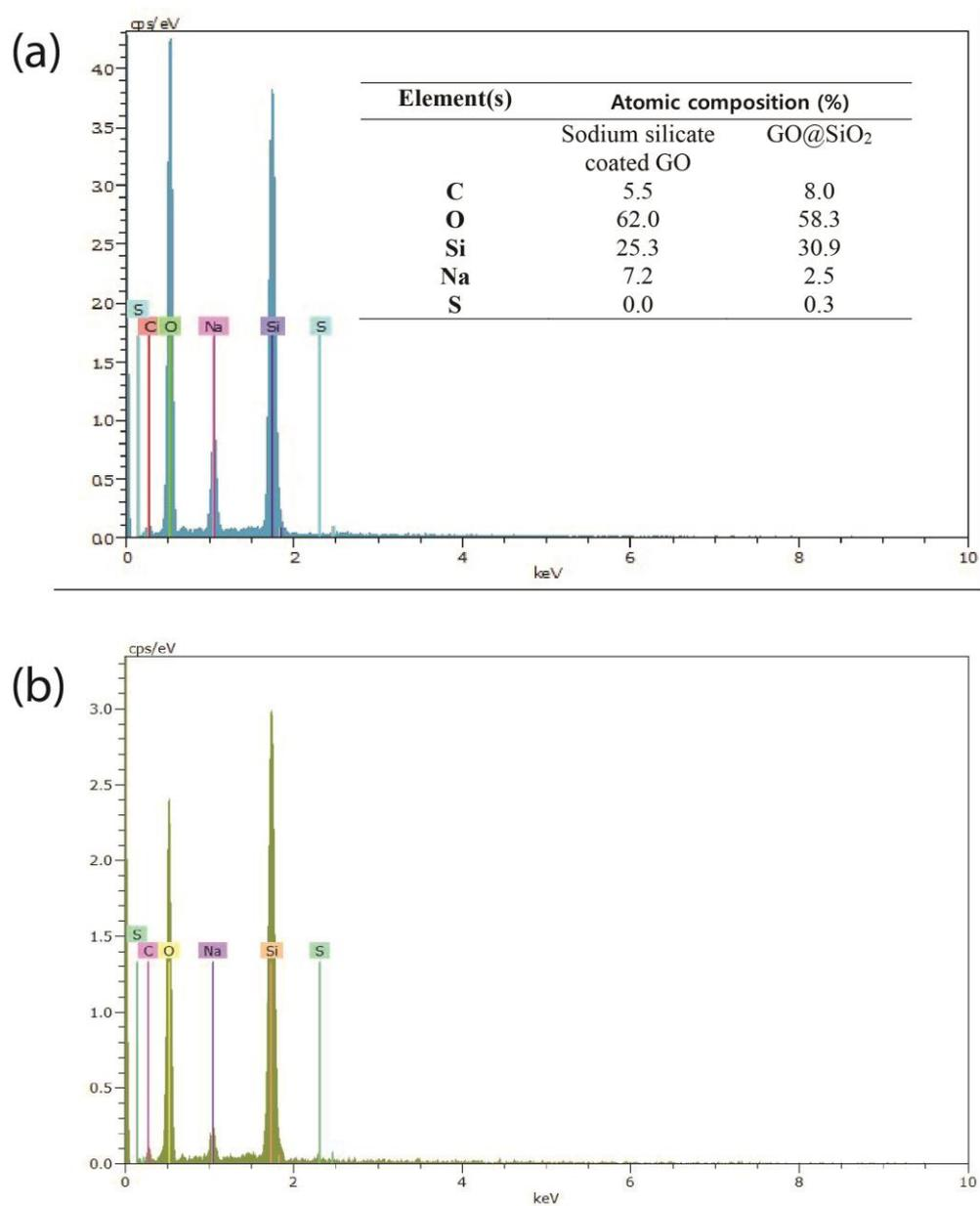
**Figure S2.** Energy dispersive X-ray spectroscopy data of (a) sodium silicate coated graphene oxide and (b) thiol functionalized silica coated graphene oxide (GO@SiO<sub>2</sub>).
