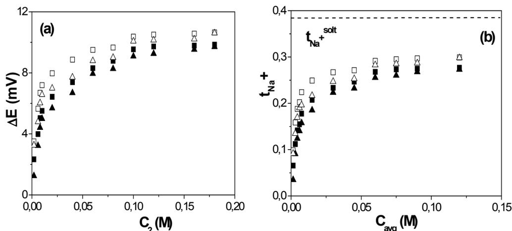
**Figure 3.** (a) Concentration potentials *versus*  $C_2$  solution concentration for the studied Al-Ox NPAM for both opposite external and solution stirring conditions; (b) Cation ( $t_+ = t_{Na^+}$ ) transport number as a function of the average concentration  $C_{avg}$ . Dense symbols: stirred solutions; open symbols: non-stirred solutions. Solution cation transport number: dot-dashed line.
