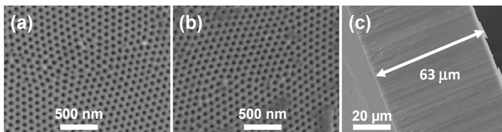
**Figure 1.** Scanning Electron Microscopy (SEM) micrographs of both membrane surfaces, (a) and (b), and cross-section (c) of the Al-Ox nanoporous alumina membrane (NPAM).
