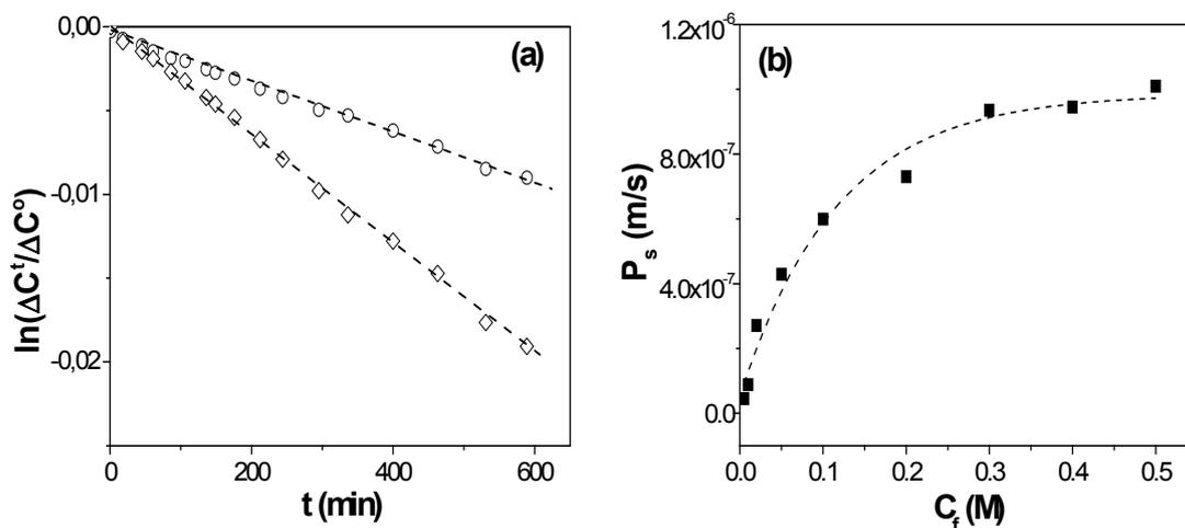
**Figure 2.** (a) Time evolution of solutions concentrations for  $C_f = 0.01$  M (o) and  $C_f = 0.1$  M (◇); (b) Variation of diffusive permeability in the membrane with NaCl feed concentration.
