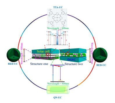
**Figure 6.** A schematic illustration of the usage of three typical upconversion materials in solar cells using two configurations. (Rare-earth upconversion, RED-UC; Upconversion in quantum nanostructure, QN-UC; Triplet-triplet annihilation upconversion, TTA-UC).
