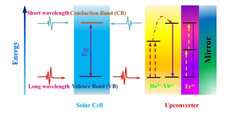
**Figure 7.** An operating mechanism for a c-Si solar cell with two upconverters, one co-doped with  $Ho^{3+}$ –Yb<sup>3+</sup> and the other one single doped with  $Er^{3+}$ . Photons with short wavelength can be absorbed directly by the solar cell. The transmitted sub-bandgap light can be upconverted into high-energy photons, which would be absorbed by c-Si. The mirror behind the upconverter increases the probability of absorption of sub-bandgap light in the upconverter layer.
