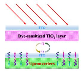
Figure 9. A typical schematic configuration of a DSSC equipped with upconverters.
