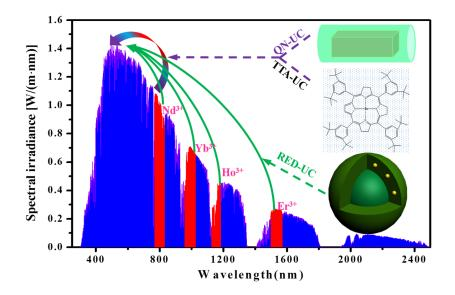
**Figure 1.** The absorption and emission range of three types of upconversion materials in reference to AM 1.5 spectrum (QN-UC (purple): upconversion in quantum nanostructures; TTA-UC (purple): triplet-triplet annihilation upconversion; RED-UC (green): Rare-earth-doped upconversion materials).
