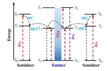
Figure 4. The working principle of the triplet-triplet annihilation upconversion.
