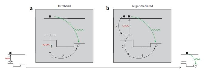
**Figure 5.** Mechanism of the upconversion in quantum nanostructures: (**a**) Direct intraband hole absorption mechanism of upconversion; (**b**) Auger-mediated upconversion (adapted with permission from [30]; Copyright Nature Publishing Group, 2013).
