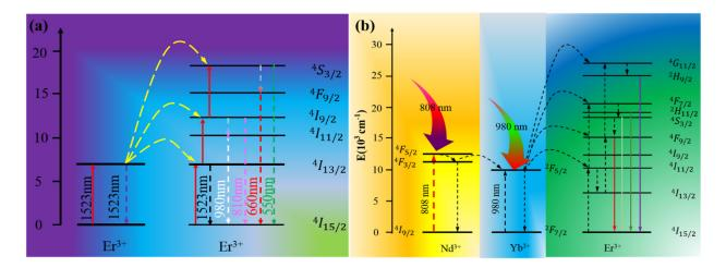
Figure 3. The upconversion mechanisms for (a) single  $Er^{3+}$  doped upconversion particles (UCNPs) excited under 1523 nm laser excitation; (b) Nd<sup>3+</sup>-Yb<sup>3+</sup>-Er<sup>3+</sup> tridoped system under 808 nm or 980 nm laser excitation.
