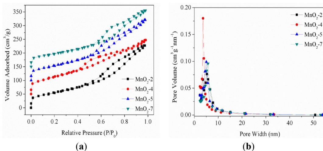
**Figure 1.** Nitrogen adsorption/desorption isotherms and BJH pore-size distribution curves of the samples MnO<sub>2</sub>-2, MnO<sub>2</sub>-4, MnO<sub>2</sub>-5, MnO<sub>2</sub>-7. **(a)** Nitrogen adsorption/desorption isotherms; **(b)** Pore-size distribution curves.
