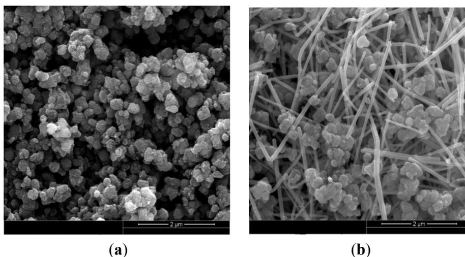
**Figure 2.** Scanning electron microscopy (SEM) images of mesoporous MnO<sub>2</sub>, mesoporous MnO<sub>2</sub>/silver nanowires. **(a)** Mesoporous MnO<sub>2</sub>; **(b)** Mesoporous MnO<sub>2</sub>/silver nanowires.
