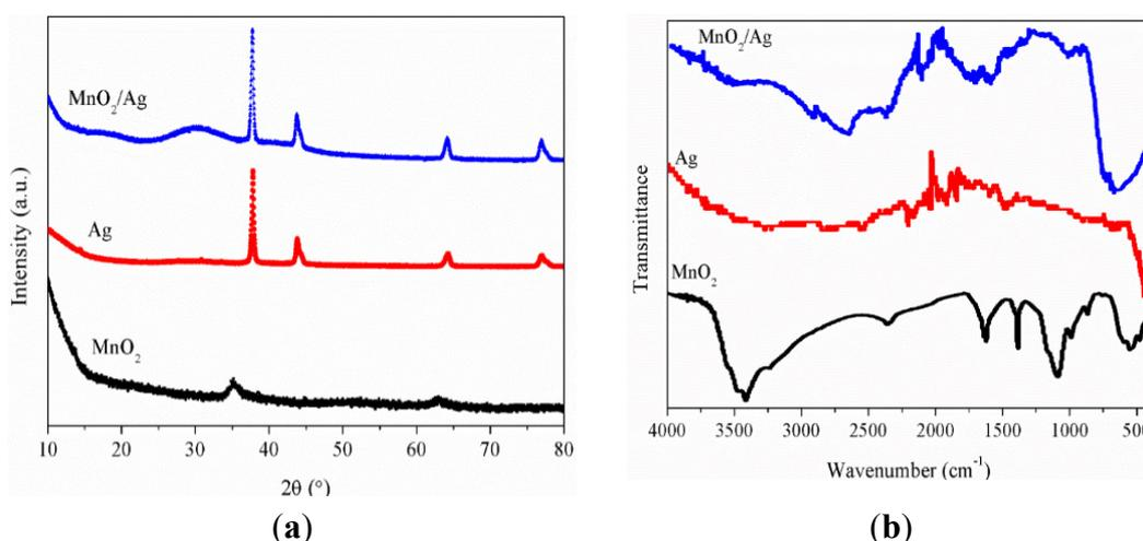
**Figure 3.** (a) X-ray diffraction (XRD) spectra of mesoporous  $\text{MnO}_2$ , silver nanowires and mesoporous  $\text{MnO}_2/\text{silver}$  nanowires; (b) Fourier transform infrared spectrometry (FT-IR) spectra of mesoporous  $\text{MnO}_2$ , silver nanowires and mesoporous  $\text{MnO}_2/\text{silver}$  nanowires.
