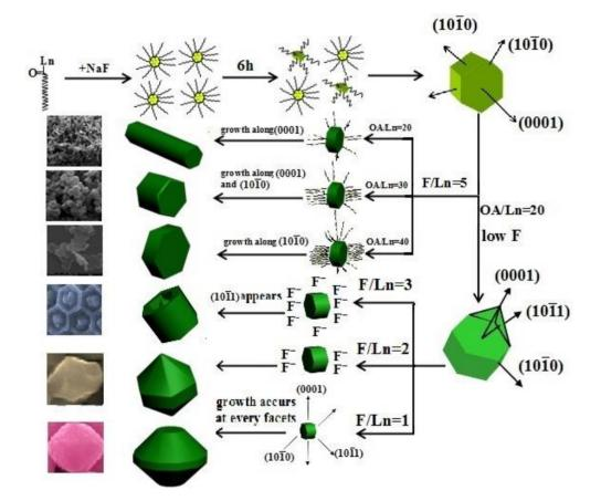
Scheme 1. Schematic illustration of the possible formation mechanism of NaYF<sub>4</sub> with various morphologies under different OA/Ln<sup>3+</sup> and  $F^-/Ln^{3+}$  molar ratio conditions.
