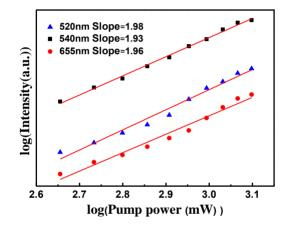
**Figure 9.** Pump power dependence of the fluorescent bands centered at 520, 540, and 655 nm from NaYF<sub>4</sub>:10% Nd<sup>3+</sup>, 10% Yb<sup>3+</sup>, 2% Er<sup>3+</sup> on pumping power.
