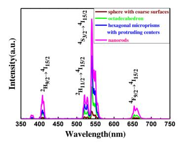
**Figure 8.** UC Photoluminescence (PL) spectra of NaYF<sub>4</sub>:10% Nd<sup>3+</sup>,10% Yb<sup>3+</sup>, 2% Er<sup>3+</sup> microcrystals with different molar ratios of  $F^-/Ln^{3+}$  (180 °C, 24 h, OA/Ln<sup>3+</sup> = 40) under diode laser excitation at 808 nm. Excitation power density, ~390 W/cm<sup>2</sup>.
