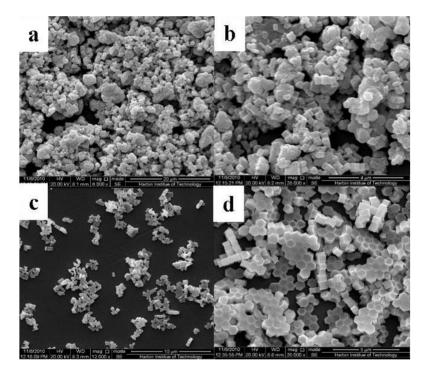
**Figure 2.** Typical field emission scanning electron microscopy (FESEM) images for the resulting NaYF<sub>4</sub>:10% Nd<sup>3+</sup>, 10% Yb<sup>3+</sup>, 2% Er<sup>3+</sup> microcrystals prepared with different hydrothermal times: (**a**) 3 h; (**b**) 6 h; (**c**) 12 h; and (**d**) 24 h (Other synthetic parameters were kept identical, 180 °C,  $F^{-}/Ln^{3+} = 5:1$ , OA/Ln<sup>3+</sup> = 40:1).
