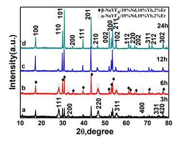
**Figure 1.** X-ray diffraction (XRD) patterns of NaYF<sub>4</sub>: 10% Nd<sup>3+</sup>,10% Yb<sup>3+</sup>, 2% Er<sup>3+</sup> microcrystals synthesized at different hydrothermal times: (**a**) 3 h; (**b**) 6 h; (**c**) 12 h; and (**d**) 24 h (180 °C  $F^-/Ln^{3+} = 5:1 \text{ OA}/Ln^{3+} = 40:1$ ).
