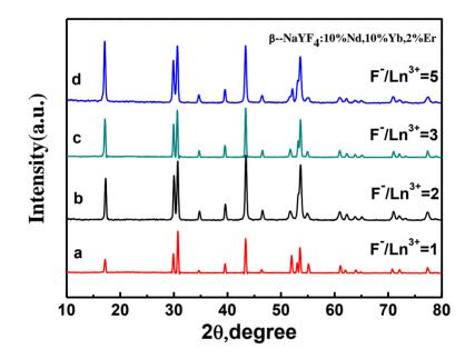
**Figure 6.** XRD patterns of NaYF<sub>4</sub>:10% Nd<sup>3+</sup>,10% Yb<sup>3+</sup>, 2% Er<sup>3+</sup> microcrystals synthesized at different molar ratios of  $F^-/Ln^{3+}$ : (a) 1:1; (b) 2:1; (c) 3:1; and (d) 5:1 (Other synthetic parameters were kept identical, 180 °C, 24 h, OA/Ln<sup>3+</sup> = 20:1).
