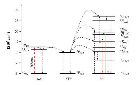
**Figure 10.** Proposed energy transfer mechanism of  $Nd^{3+}$ ,  $Yb^{3+}$ ,  $Er^{3+}$  ions following diode laser excitation of 808 nm. The dashed-dotted, dashed, dotted, and full arrows represent the photon excitation, energy transfer, and emission processes.
