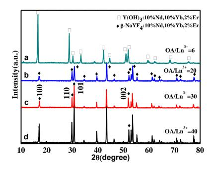
**Figure 4.** XRD patterns of NaYF<sub>4</sub>:10% Nd<sup>3+</sup>, 10% Yb<sup>3+</sup>, 2% Er<sup>3+</sup> microcrystals synthesized at different molar ratios of OA/Ln<sup>3+</sup>: (**a**) 6:1; (**b**) 20:1; (**c**) 3:1; and (**d**) 40:1 (Other synthetic parameters were kept identical, 180 °C, 24 h,  $F^-/Ln^{3+} = 5:1$ ).
