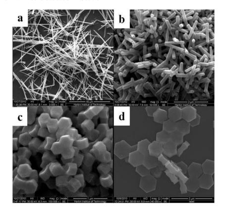
**Figure 3.** Typical FESEM images for the as-prepared NaYF<sub>4</sub>: 10% Nd<sup>3+</sup>,10% Yb<sup>3+</sup>, 2% Er<sup>3+</sup> microcrystals at different molar ratios of OA/Ln<sup>3+</sup>: (**a**) 6:1; (**b**) 20:1; (**c**) 30:1; and (**d**) 40:1 (Other synthetic parameters were kept identical, 180 °C, 24 h,  $F^-/Ln^{3+} = 5:1$ ).
