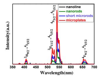
**Figure 7.** UC Photoluminescence (PL) spectra of NaYF<sub>4</sub>:10% Nd<sup>3+</sup>,10% Yb<sup>3+</sup>, 2% Er<sup>3+</sup> microcrystals with different molar ratios of OA/Ln<sup>3+</sup> under diode laser excitation at 808 nm. Excitation power density, ~390 W/cm<sup>2</sup>.
