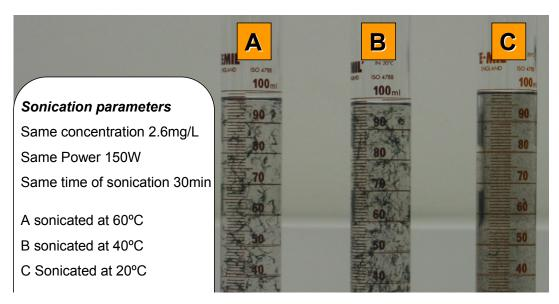
Furthermore the shape of the macro bundles formed in the three decanted suspensions is clearly different (Figure 6). The bundles formed at the higher temperature appear more loosely bundled and more filamentous compared to the tightly packed bundles seen in the original solutions. A video showing snapshots of a 6 h decanting test is also provided in the supplementary information.
