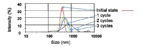
Figure 8. Improvement of the CNT dispersion after three freezing cycles at -17 °C. (A) and (B) represent a 2.6 mg/L suspension before and after the three bath cryo-sonication cycles, respectively.
