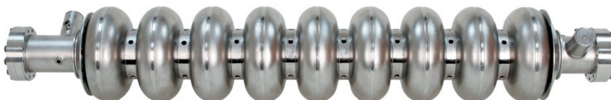
Figure 1. Niobium SRF cavity. Reproduced from the Fermilab SRF Materials Research Department [4].
