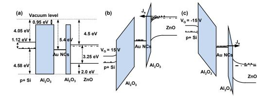
Figure 6. Band diagram of proposed ZnO TFT memory. (a) flatband; (b) programming; (c) erasing.
