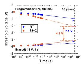
Figure 7. Retention characteristics of fabricated ZnO TFT memory under RT and 85 °C.
