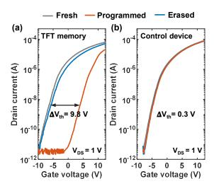
**Figure 4.** (a,b) Transfer curve of TFT memory and control device at fresh state, after 15 V, 100 ms programming and after -15 V, 1 s erasing.
