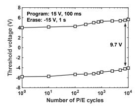
Figure 8. Endurance characteristics of fabricated ZnO TFT NCs memory.
