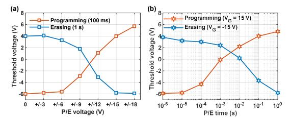
Figure 5. P/E characteristics of TFT memory. (a) V<sub>th</sub> versus P/E voltage; (b) V<sub>th</sub> versus P/E time.
