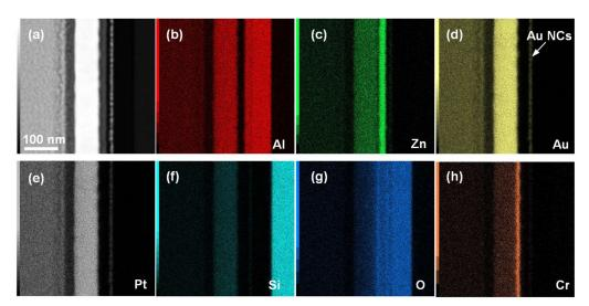
**Figure 2.** (a) Annular dark field image of the fabricated TFT memory; (b–h) EDS mapping profiles in the drain region, showing the distribution of Al, Zn, Au, Pt, Cr, Si, and O elements.
