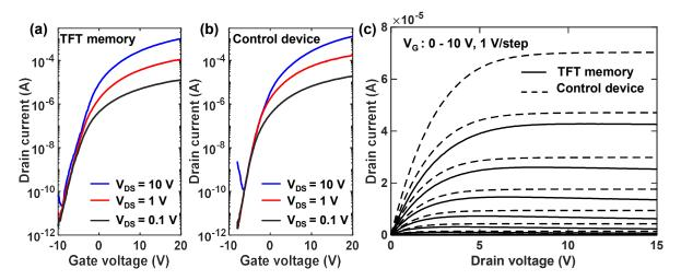
**Figure 3.** (a,b) Transfer curves of fabricated TFT memory and control device; (c) output curves of fabricated TFT memory and control device.
