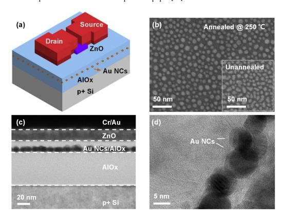
**Figure 1.** (a) Schematic of the proposed TFT memory; (b) SEM image of Au NCs on AlO<sub>x</sub> blocking oxide after annealing, insert is the SEM image of the unannealed sample; (c) cross-sectional TEM image of the fabricated TFT memory; (d) high-resolution TEM image of Au NCs in the TFT memory.
