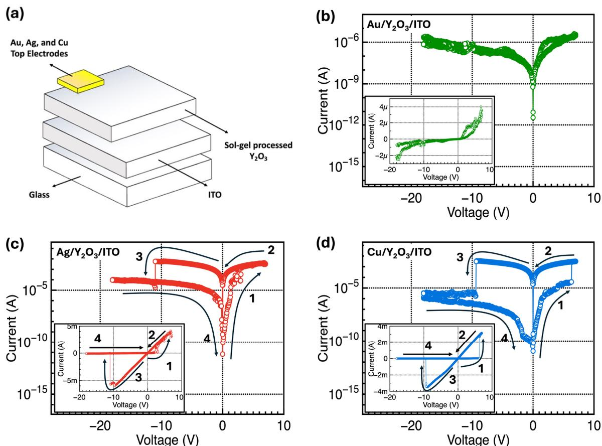
**Figure 4.** (a) Schematic of the fabricated  $Y_2O_3$ -based RRAM devices and (b–d) representative I–V curves of the  $Y_2O_3$ -based stacked-structure RRAM devices with different TEs.
