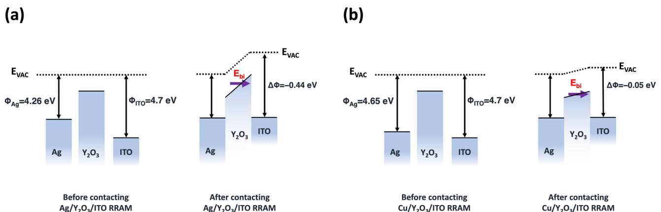
**Figure 6.** Energy diagrams for (a) Ag/Y<sub>2</sub>O<sub>3</sub>/ITO and (b) Cu/Y<sub>2</sub>O<sub>3</sub>/ITO RRAM devices, before and after contact.
