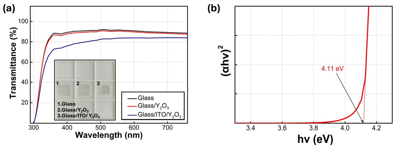
**Figure 3.** (a) Transmittance spectra of bare glass, glass/ $\text{Y}_2\text{O}_3$  films and the glass/ITO/ $\text{Y}_2\text{O}_3$ ; the inset shows the optical images of the films. (b)  $(\alpha h\nu)^2$ -versus- $h\nu$  plot of the  $\text{Y}_2\text{O}_3$  films.
