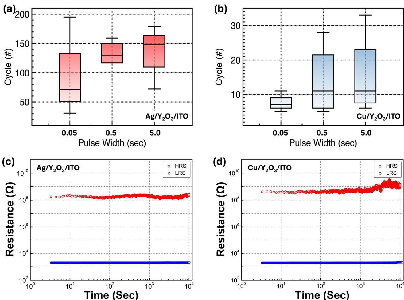
**Figure 7.** Endurance test results as a function of pulse width: (a) ITO/Y<sub>2</sub>O<sub>3</sub>/Ag and (b) ITO/Y<sub>2</sub>O<sub>3</sub>/Cu RRAM devices as a function of pulse widths. Retention test results: (c) ITO/Y<sub>2</sub>O<sub>3</sub>/Ag and (d) ITO/Y<sub>2</sub>O<sub>3</sub>/Cu RRAM devices, after the programming and erase operations (each pulse width: 50 ms).
