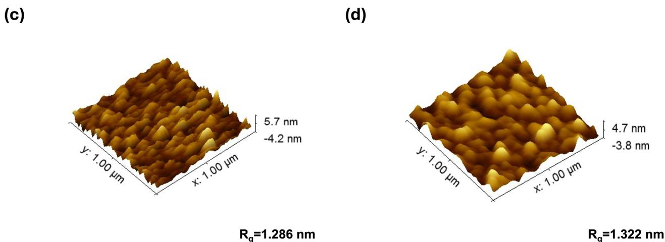
**Figure 1.** (a) GIXRD spectra and (b) the cross-sectional SEM image of  $Y_2O_3$  film. Three-dimensional SPM surface images of the ITO/glass substrates, (c) and a sol-gel-processed  $Y_2O_3$  film on ITO/glass substrates (d), respectively.
