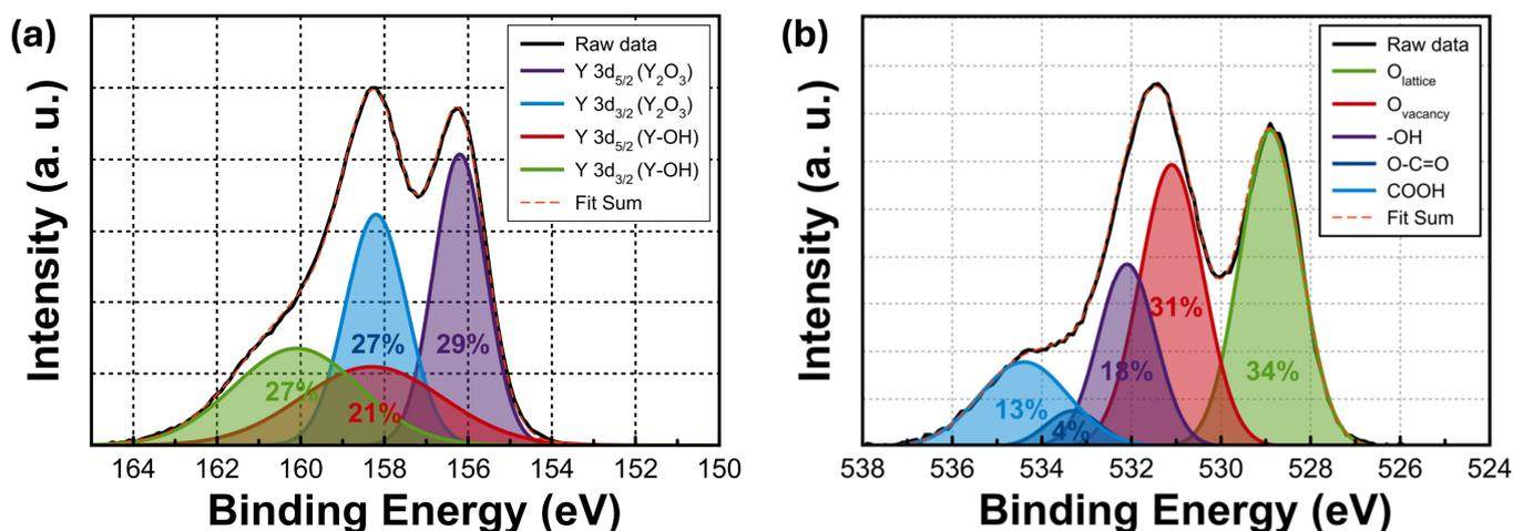
**Figure 2.** XPS curves of (a) Y3d and (b) O1s for the sol-gel-processed  $Y_2O_3$  films.
