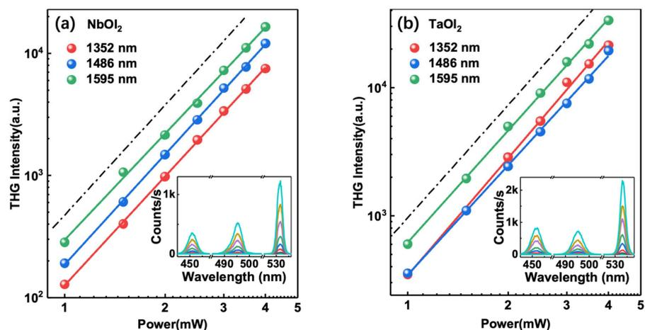
**Figure 2.** Fundamental power dependence of THG signal for (a) NbOI<sub>2</sub> and (b) TaOI<sub>2</sub> excitation at 1352, 1486, and 1595 nm. The black dot dashed line serves as a guide for a slope of  $\sim 3$ . The inset illustrates the power dependence THG spectra for NbOI<sub>2</sub> and TaOI<sub>2</sub> under the three excitation wavelengths. The excitation average powers changes from 1 to 4 mW corresponds to the line color of black to cyan.
