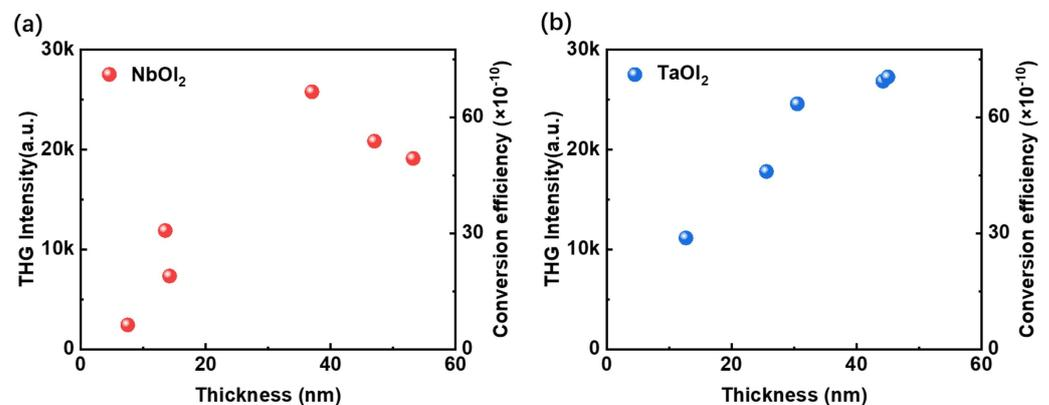
**Figure 5.** THG responses and conversion efficiency as a function of thickness. (a) NbOI<sub>2</sub> and (b) TaOI<sub>2</sub> with a thickness range of 7.5 to 53.2 nm and 12.7 to 45 nm, respectively.
