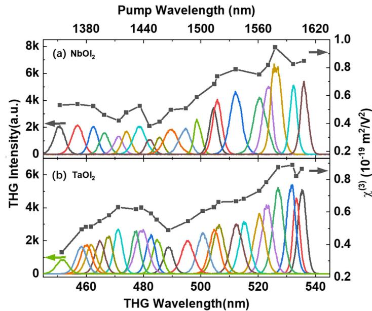
**Figure 4.** THG emission spectroscopy (left panel, spectra in colorful lines, guided by left arrows) and third-order nonlinear susceptibility  $\chi^{(3)}$  (right panel, black squares, guided by right arrows) of (a) 22 nm-NbOI<sub>2</sub> and (b) 20 nm-TaOI<sub>2</sub> at the fundamental excitation wavelength range of 1350 to 1605 nm. All the measurements were taken with the same average excitation power. Top panel corresponds to the fundamental excitation wavelength.
