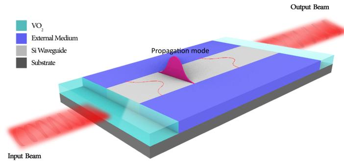
**Figure 1.** A 3D schematic of the proposed RI resonator.
