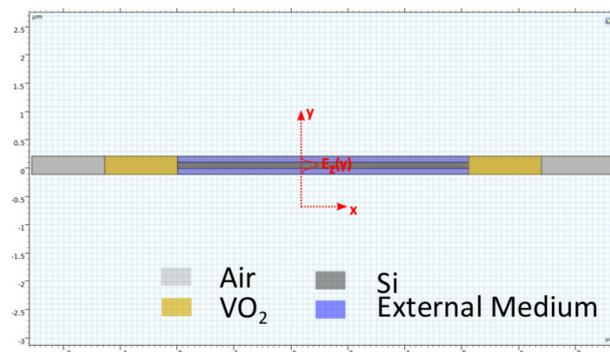
**Figure 2.** The proposed linear resonator model for RI sensing in COMSOL Multiphysics environment with the different colored regions defining Si waveguide,  $\text{VO}_2$ , air and external medium. Similarly, the direction of light propagation is in the z-direction.
