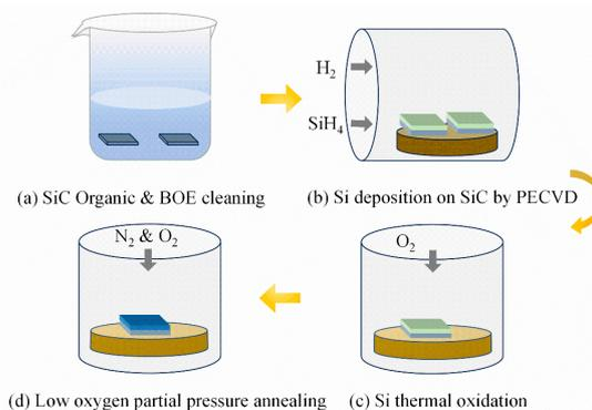
**Figure 1.** Schematic diagram of  $SiO_2/SiC$  structure formation and annealing process.
