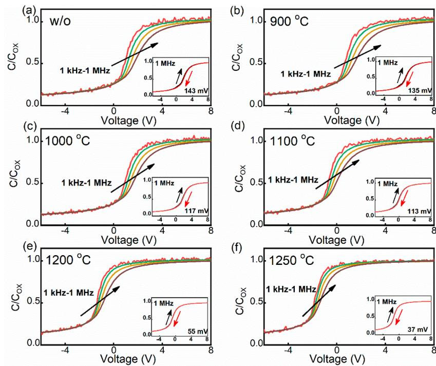
**Figure 3.** The multi-frequency C-V curves from 1 kHz to 1 MHz for the samples (a) without annealing and with annealing at (b) 900 °C, (c) 1000 °C, (d) 1100 °C, (e) 1200 °C, and (f) 1250 °C. Bidirectional C-V curves measured at 1 MHz are shown in the inset.
