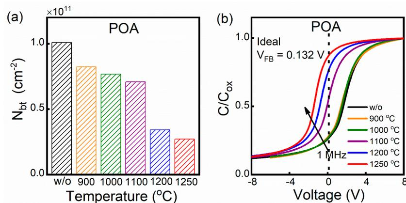
**Figure 5.** (a) Border trap density ( $N_{bt}$ ) and (b) 1 MHz C-V curves of annealed samples at different temperatures.
