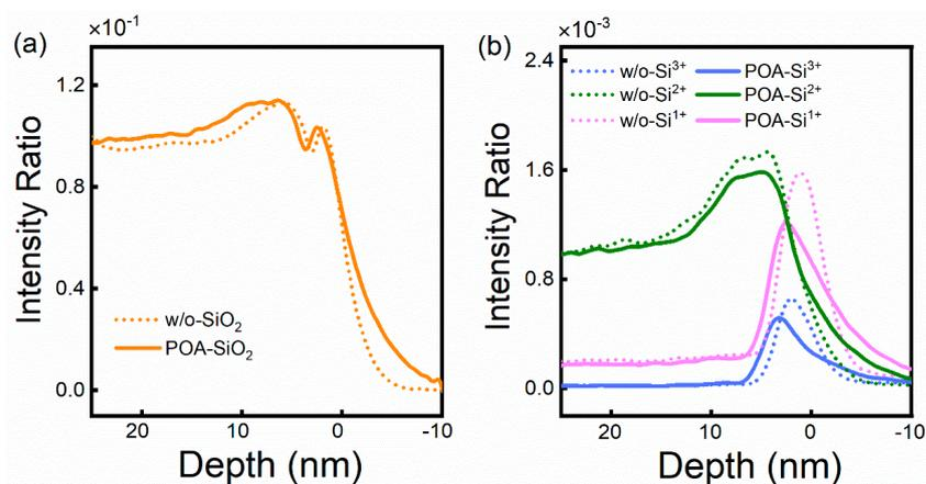
**Figure 7.** The depth distribution of oxides corresponding to the valence states (a)  $\text{Si}^{4+}$ , (b)  $\text{Si}^{3+}$ ,  $\text{Si}^{2+}$ , and  $\text{Si}^{1+}$  of Si, respectively.
