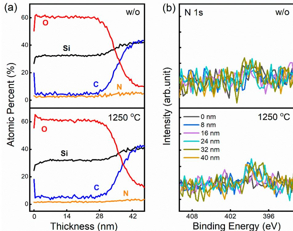
**Figure 2.** (a) The atomic percent of Si, O, C, and N elements and (b) the N 1s peak of the samples without and with annealing at 1250 °C.
