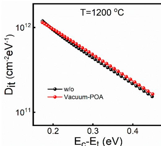
**Figure 6.** The  $D_{it}$  of the samples without and with annealing in vacuum at 1200 °C.
