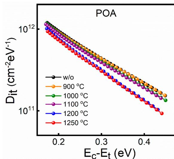
**Figure 4.** The  $D_{it}$  calculated by the high–low method for the sample annealed from 900 to 1250 °C, respectively.
