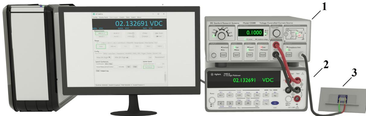
**Figure 6.** The experimental setup for studying conductivity evolution in the ensembles of anatase inter-electrode bridges; 1—voltage-controlled current source; 2—multimeter; 3—sample under study.
