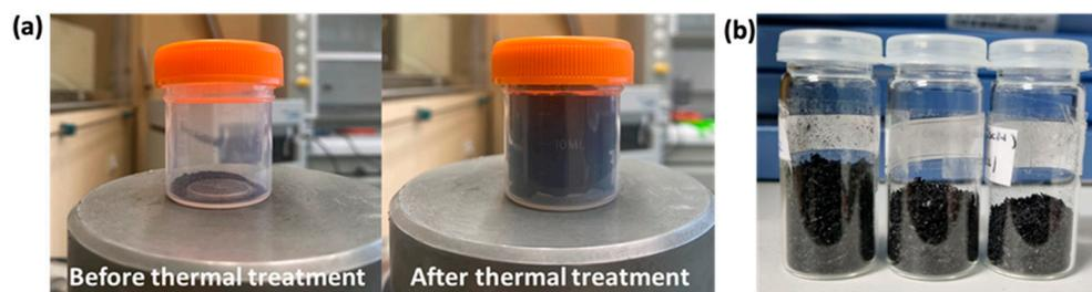
**Figure 2.** (a) Picture of the GO powder before reduction (left) and after reduction (right) using HP treatment. (b) Picture of LrGO material after reduction of GO powder using CO<sub>2</sub> laser irradiation. Each bottle, from left to right, contains the rGO obtained by applying a power of 1.6 W, 1.8 W and 2.0 W.
