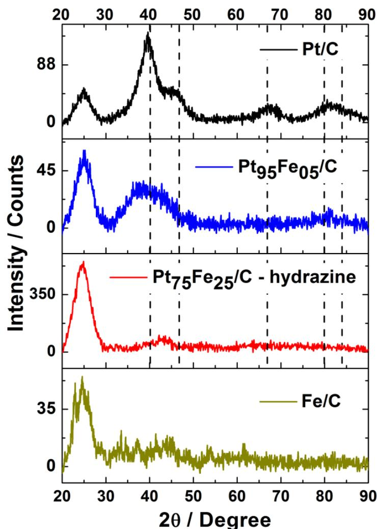
**Figure 2.** XRD patterns of the Pt and PtFe-based electrocatalysts.
