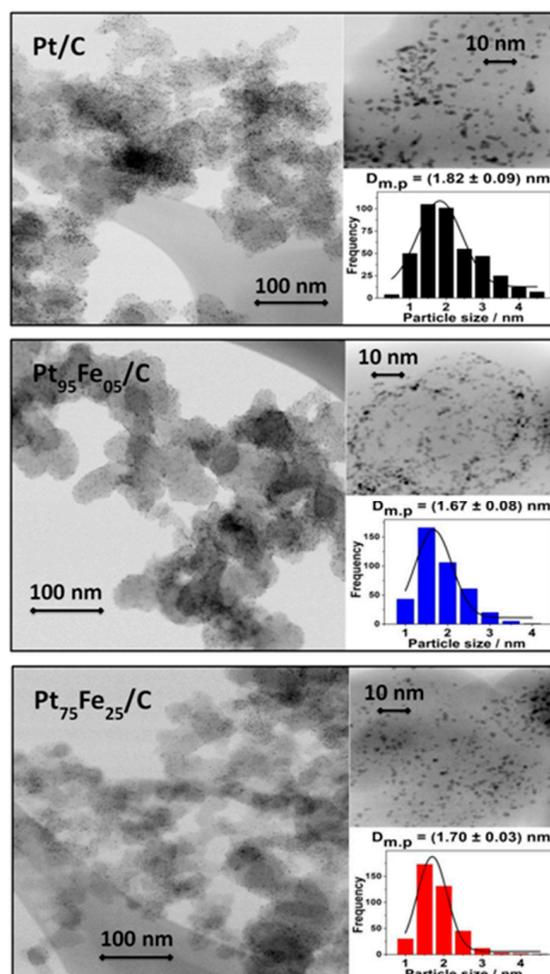
**Figure 3.** TEM images and histograms of the carbon-supported Pt and PtFe nanomaterials synthesized by the polyol method. Count: 400 particles.
