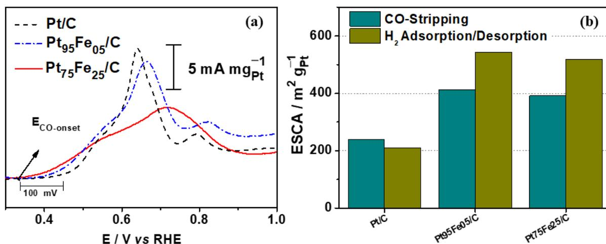
**Figure 6.** (a) CO stripping voltammogram for the platinum-based electrocatalysts in alkaline medium; (b) comparison of ECSA obtained by CO stripping and H<sub>2</sub> adsorption/desorption experiments.
