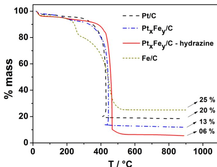
**Figure 1.** Thermogravimetric analysis curves of the Fe/C, Pt/C, and Pt<sub>x</sub>Fe<sub>y</sub>/C electrocatalysts under compressed air atmosphere recorded at 10 °C min<sup>-1</sup>.
