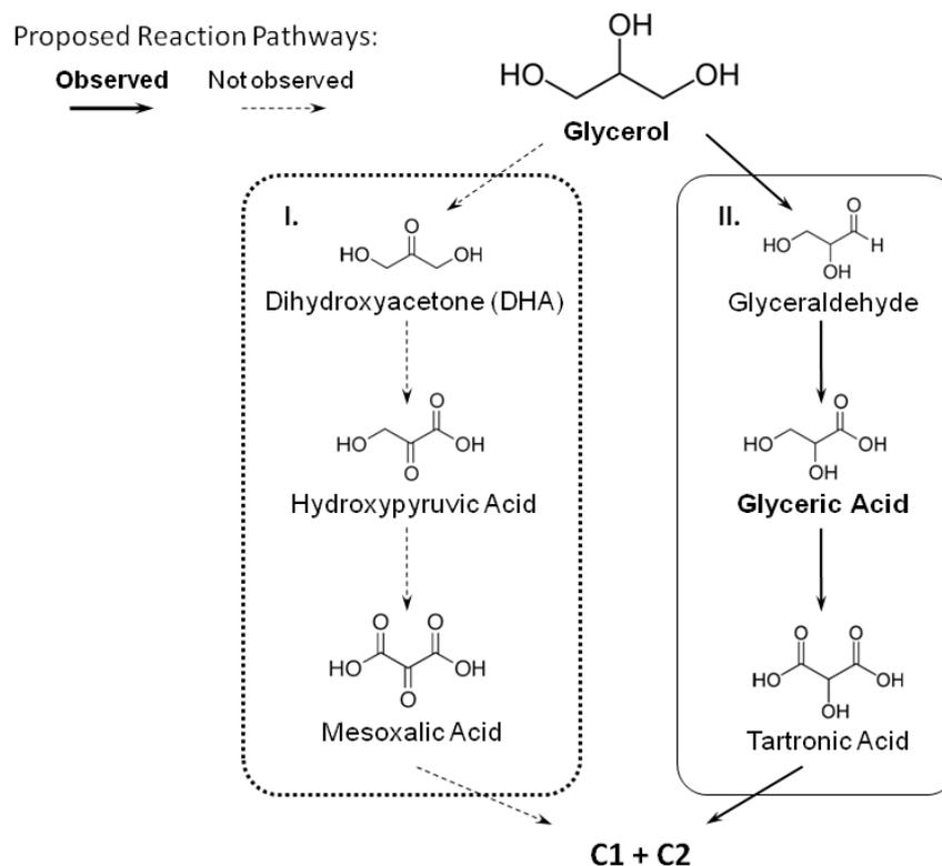
**Figure 8.** Proposed mechanism for glycerol electro-oxidation vs. that of Pt<sub>75</sub>Fe<sub>25</sub>/C.
