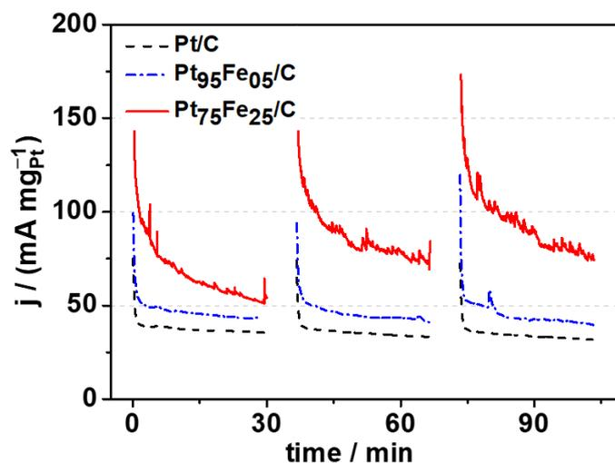
Figure 5. Chronoamperometric curves of the PtFe/C electrocatalyst for glycerol electro-oxidation ( $0.5 \text{ mol L}^{-1}$ ). Supporting electrolyte NaOH  $0.1 \text{ mol L}^{-1}$ ,  $E_{\text{app}} = +0.7 \text{ V vs. RHE}$ .
