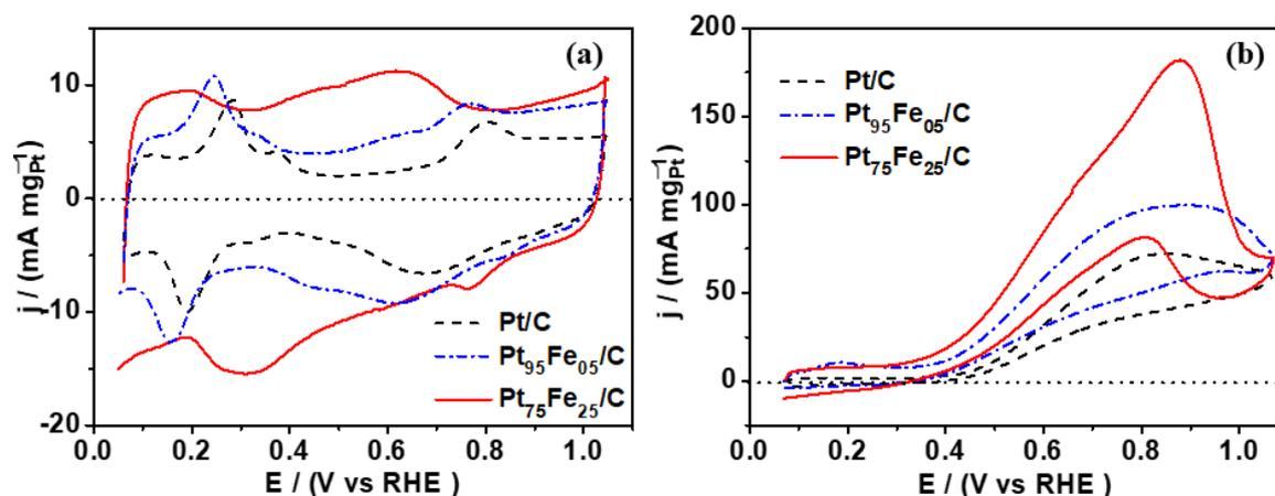
**Figure 4.** Cyclic voltammogram of platinum-based electrocatalysts in (a) NaOH 0.1 mol L<sup>-1</sup> and (b) NaOH 0.1 mol L<sup>-1</sup> + Glycerol 0.5 mol L<sup>-1</sup>.
