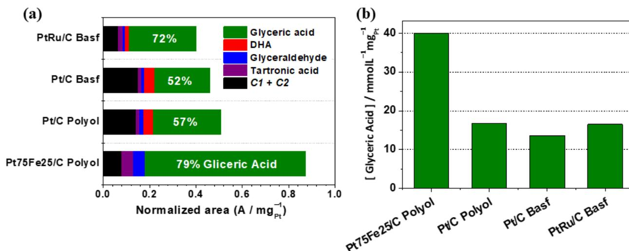
**Figure 7.** (a) Distribution of the glycerol electro-oxidation products as a function of time at +0.7 V vs. RHE at 4 h on the platinum-based electrocatalysts in 0.1 mol L<sup>-1</sup> NaOH + 0.5 mol L<sup>-1</sup> glycerol. (b) Concentration glyceric acid normalized per mg of platinum.
