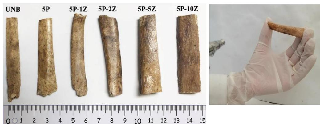
**Figure 3.** Airbrushed PSF/ZnO historical bone samples as a function of particle content (**Left**) and a photograph of the airbrushing process on the surface of historical bone (**Right**).
