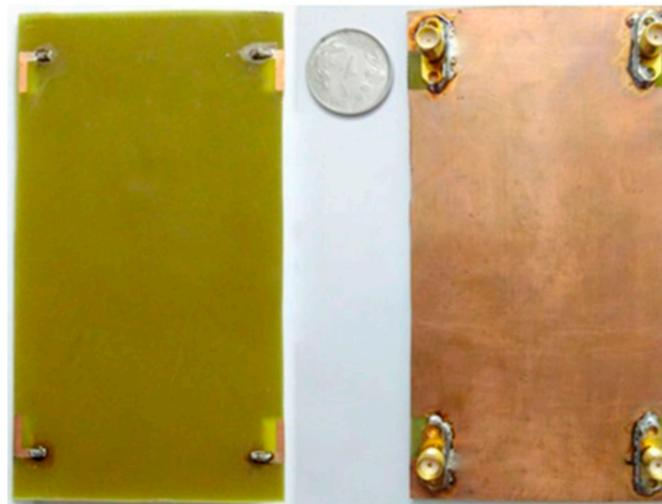
**Figure 23.** Front and back plane of the fabricated L-shaped and ground plane with four etched slots for the  $(4 \times 4)$  MIMO antenna [106].
