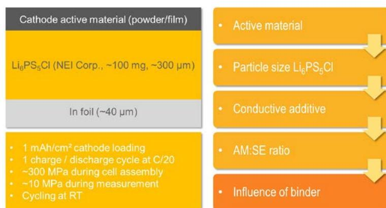
**Figure 1.** Schematic outline of the composite cathode optimization by dry- and wet-chemical processing. In addition, the testing conditions are listed.
