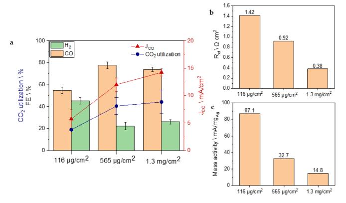
**Figure 4.** (a) FE, CO<sub>2</sub> utilization, and CO partial current density for different silver mass-loadings:  $116 \mu g/cm^2$  (sample D),  $565 \mu g/cm^2$  (sample B), and  $1.13 mg/cm^2$  (sample E). (b) Values of R<sub>ct</sub> that emerged from the EIS analysis. (c) Values of mass activity for each sample.
