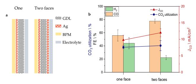
**Figure 2.** (a) Schematic representation of the GDEs with silver sputtered on one face (sample A) and both (sample B) faces. (b) FE, CO<sub>2</sub> utilization and CO partial current density obtained by the two GDEs samples.
