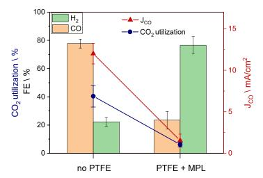
**Figure 3.** FE, CO<sub>2</sub> utilization, and CO partial current density obtained with GDEs with two different GDLs: one has not been treated with PTFE and does not include an MPL (sample B), while the other has a strong hydrophobic feature thanks to the PTFE and MPL (sample C).
