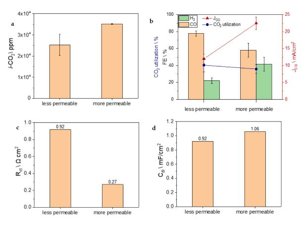
**Figure 6.** (a) Concentration of i-CO $_2$  produced by the electrolyzer using carbon supports with different permeability: less permeable (sample B) and more permeable (sample F). (b) FE, CO $_2$  utilization, and partial current density for CO. (c) Charge transfer resistance values and (d) double-layer capacitance values obtained by EIS analysis.
