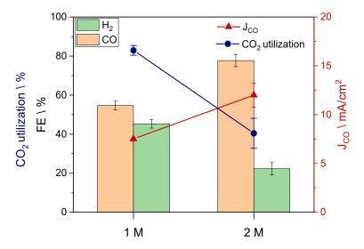
**Figure 5.** FE, CO<sub>2</sub> utilization, and CO partial current density when varying the concentration of the bicarbonate solution. GDE sample: B.
