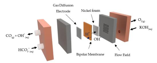
Figure 1. Schematic representation of the bicarbonate MEA electrolyzer.
