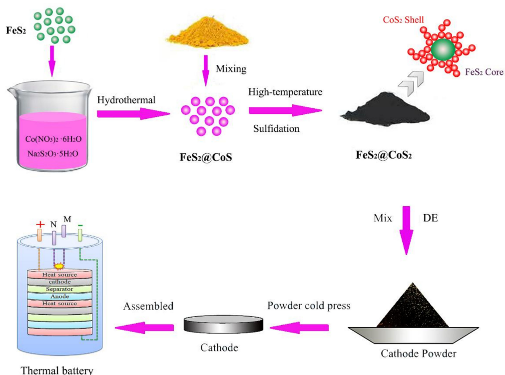
Figure 1. Schematics showing the synthesis process of the \text{FeS}_2@\text{CoS}_2 and battery assembly.
