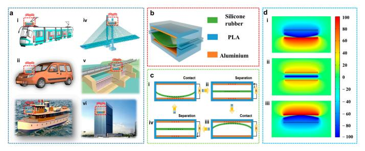
**Figure 1.** Application scenario, structure and working principle of SRS-TENG. (a) SRS-TENG application in various scenarios, such as (i) metro, (ii) vehicle, (iii) ship, (iv) bridge, (v) hydroelectric power plant, and (vi) building. (b) The structure and (c) (i–iv) working mechanism of the SRS-TENG; (d) (i–iii) the potential distribution of two parallel electrodes at different states calculated by COMSOL Multiphysics (COMSOL Inc., Stockholm, Sweden).
