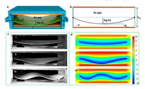
**Figure 2.** Analysis of the movement of silicone rubber strip. (a) The coordinate system of the SRS-TENG shown in the 3D structure; (b) parameters of the SRS-TENG; (c) silicone rubber strip taken by high-speed camera and (d) its corresponding simulation result by COMSOL Multiphysics at vibration frequencies of (i) 10 Hz, (ii) 30 Hz and (iii) 50 Hz, respectively.
