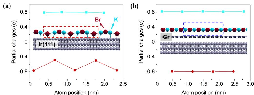
**Figure 2.** Simulated model (lateral view) of both KBr structures with the partial charges in the dotted box of the model calculated by the Bader method (K in blue, Br in red, C in black and Ir in gray): (a) KBr/Ir(111), (b) KBr/Gr/Ir(111).
