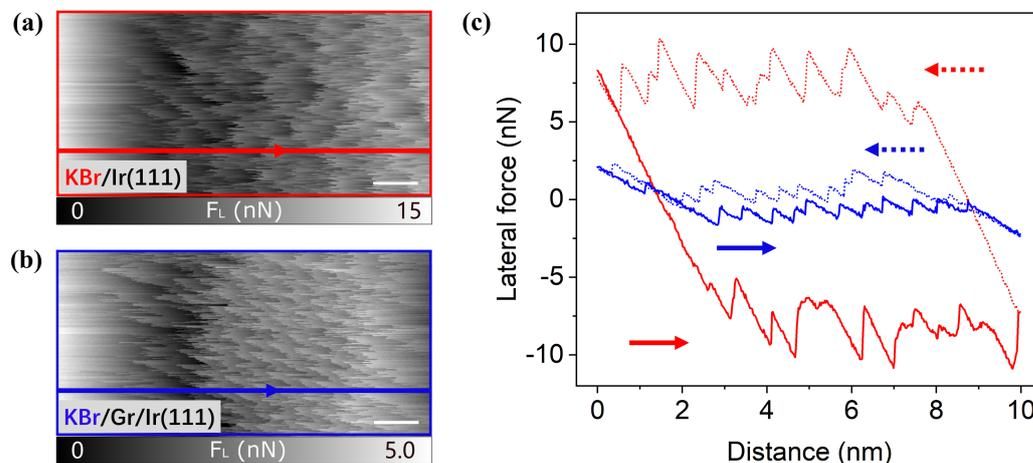
**Figure 3.** Frictional images (forward direction of the two KBr structures at a normal load of  $F_n = 5$  nN: (a) KBr/Ir(111), (b) KBr/Gr/Ir(111). Scale bar: 1 nm. The corresponding friction loops of a single line marked in both images are presented in (c).
