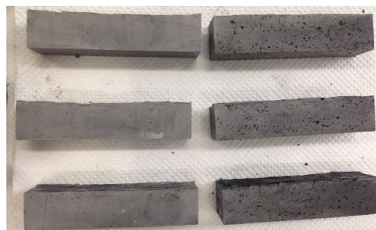
**Figure 7.** MWCNT/white cement mortar specimens dispersed with the superplasticizer on the left and the SDBS surfactant on the right.
