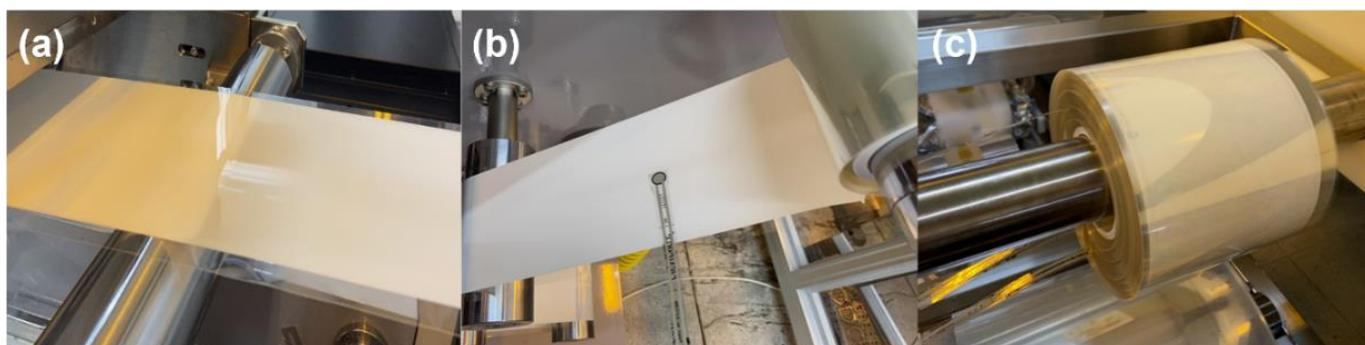
**Figure 3.** (a) Gadolinium-doped ceria coating layer; (b) the force-sensing resistor at the rewinding section; and (c) wound coated layer aging procedure.
