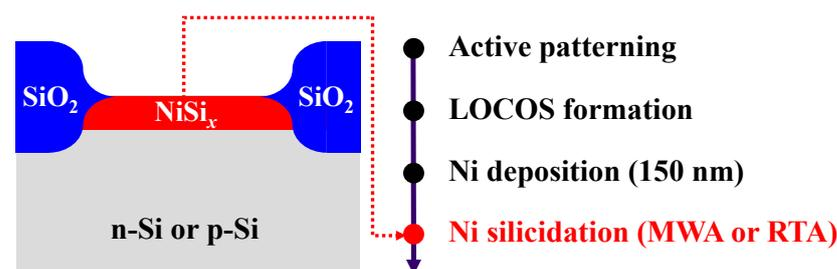
**Figure 2.** The schematic structure and process flow of the NiSi<sub>x</sub> SB-diodes.
