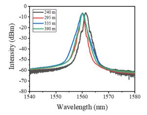
Figure 9. Optical spectra at the maximum output power level of the four cavities with different lengths.
