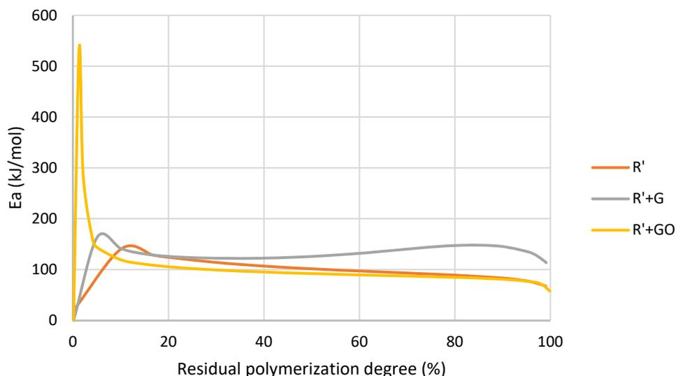
Figure 12. Activation energy as a function of residual conversion degree of R' and R'+GBN after UV exposure obtained by MFK model.
