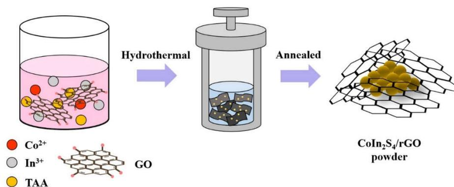
**Scheme 1.** Preparation process of CoIn<sub>2</sub>S<sub>4</sub>/C composite.
