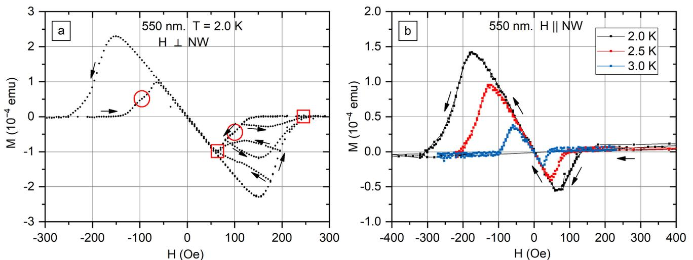
**Figure 6.** The magnetic moment  $M$  of 550-nm-diameter In nanowire array as a function of transverse (a) and axial (b) magnetic field  $H$ . Arrows show how the field was changing. Two joining points of minor loops are marked with red squares. The feature of the  $M(H)$  curve in the transverse field, which is absent in case of axial field, is marked with the red circle in panel (a).
