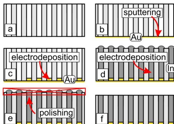
**Figure 2.** A flowchart of In nanowire array preparation process. (a) The original porous template. (b) Sputtering of Au layer on the porous template. (c) Templated electrodeposition of short Au nanorods. (d) Templated electrodeposition of In until complete filling of the pores by the metal. (e) Mechanical polishing of the top part of the nanocomposite to remove In from sample surface. (f) Resulting nanocomposite.
