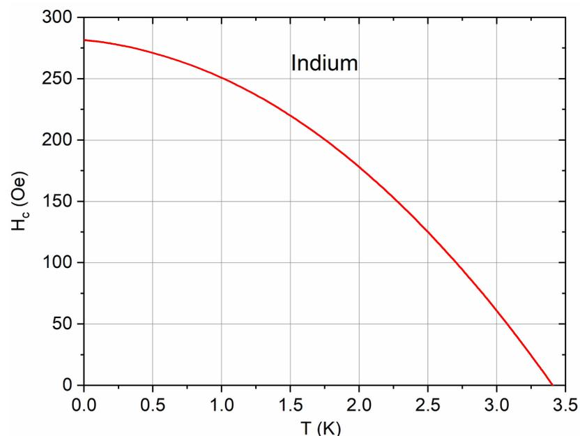
**Figure A1.** Experimental measurement of the critical field in bulk In as a function of temperature [30].
