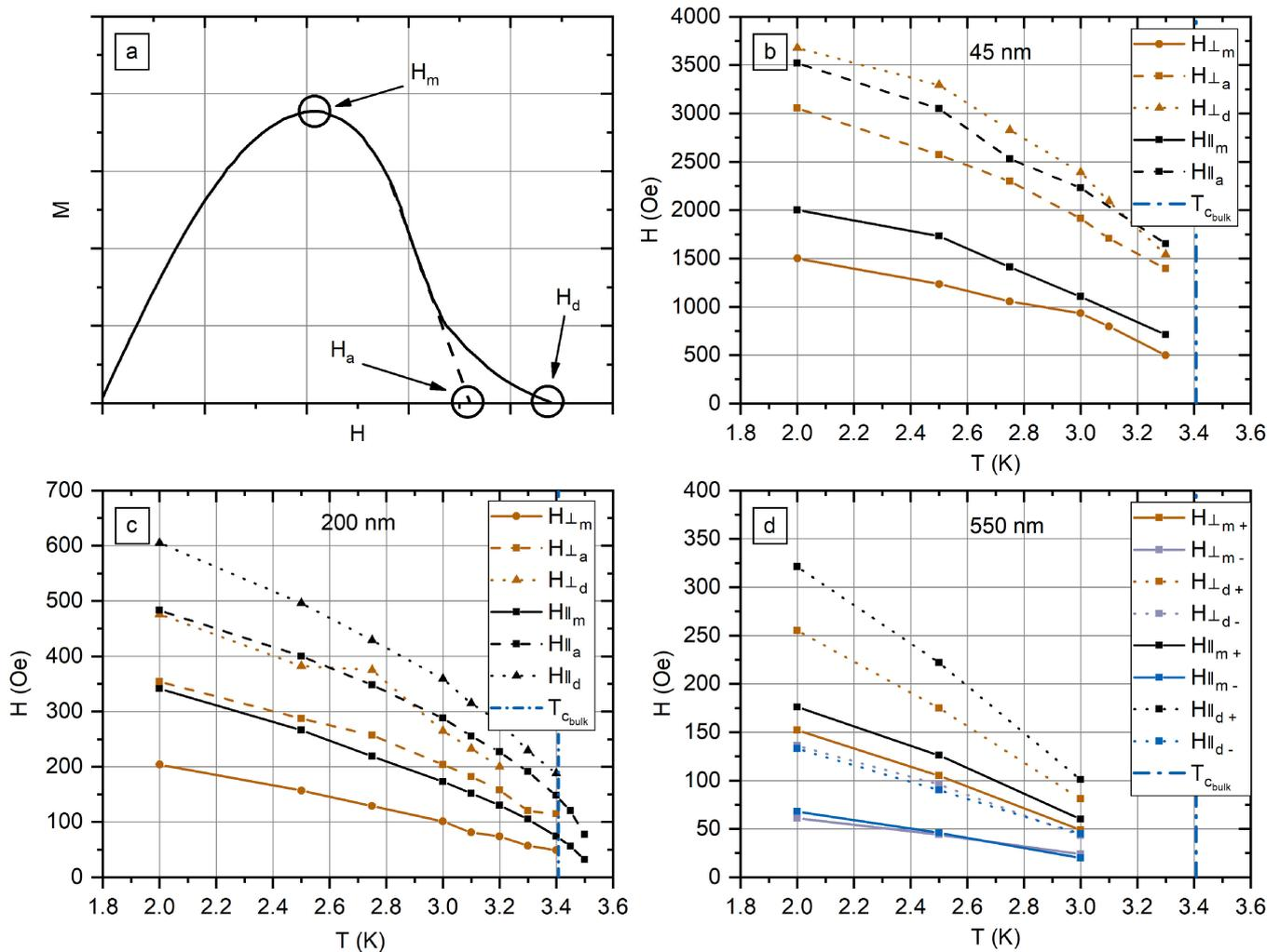
**Figure 7.** (a) Schematic illustration of the critical fields  $H_m$ ,  $H_a$ , and  $H_d$  on  $M(H)$  curve. Values of fields measured for the arrays of In nanowires with a diameter of 45 nm (b), 200 nm (c), and 550 nm (d). Values measured for increasing in modulus field  $H$  have index +, whereas values measured for decreasing in modulus field  $H$  have index –.
