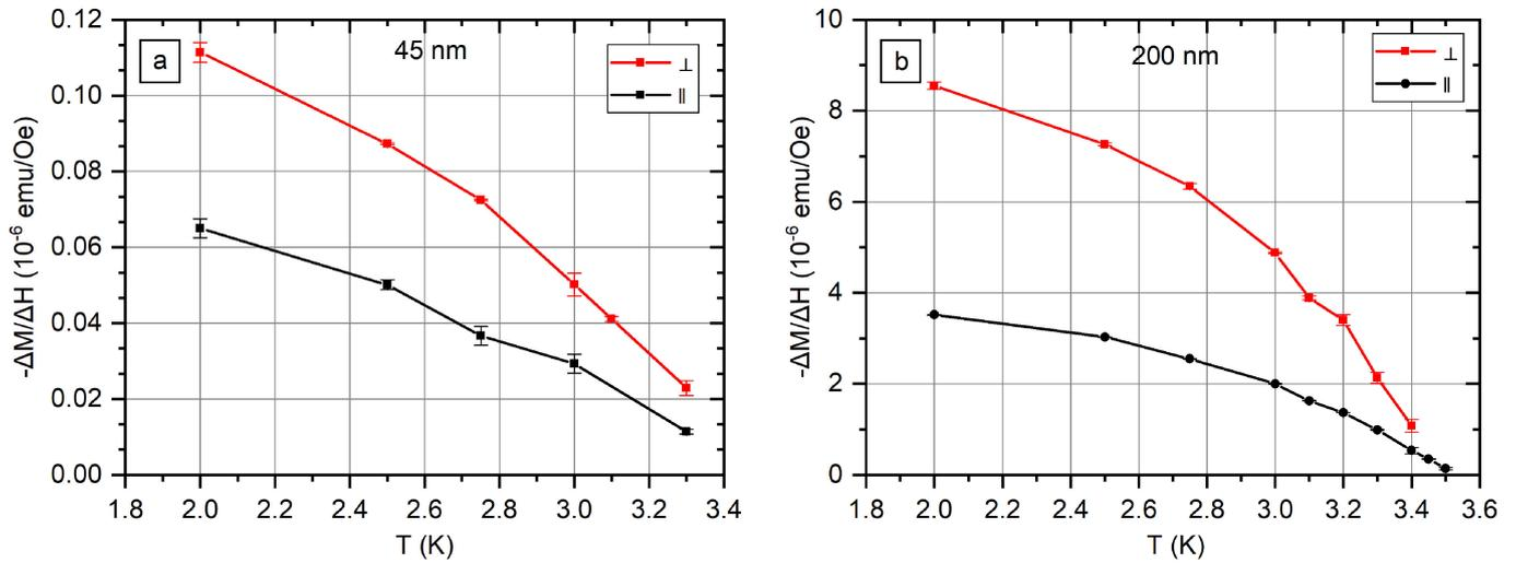
**Figure 8.** The slope of the linear part of  $M(H)$  curve observed at small fields for s45 (a) and s200 (b).
