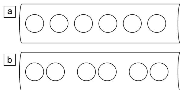
**Figure 1.** Scheme of the simplest possible vortex configurations in nanowire according to the simulation [24]: 1D lattice of single-quantum vortices (a) and a row of single-quantum vortices divided into pairs (b). Circles are superconducting vortices.
