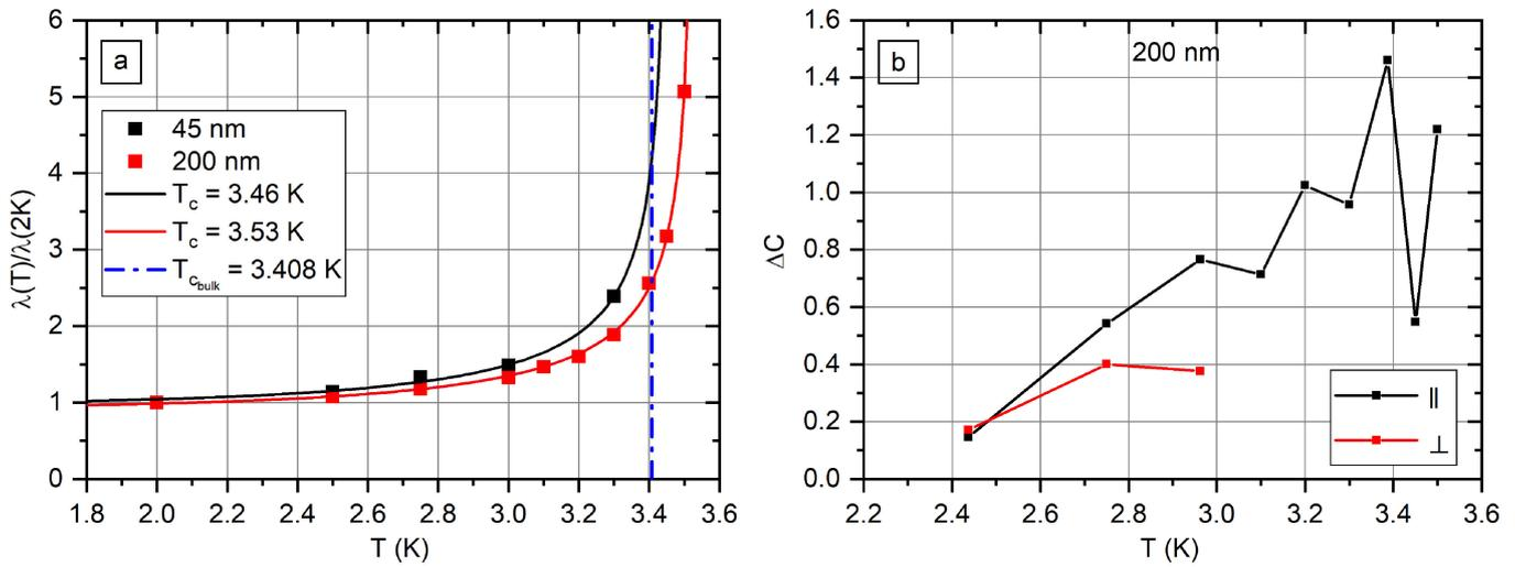
**Figure 9.** Magnetic field penetration depth as a function of temperature (a). The difference in heat capacities  $\Delta C$  of the normal and the superconducting states as a function of temperature (b).
