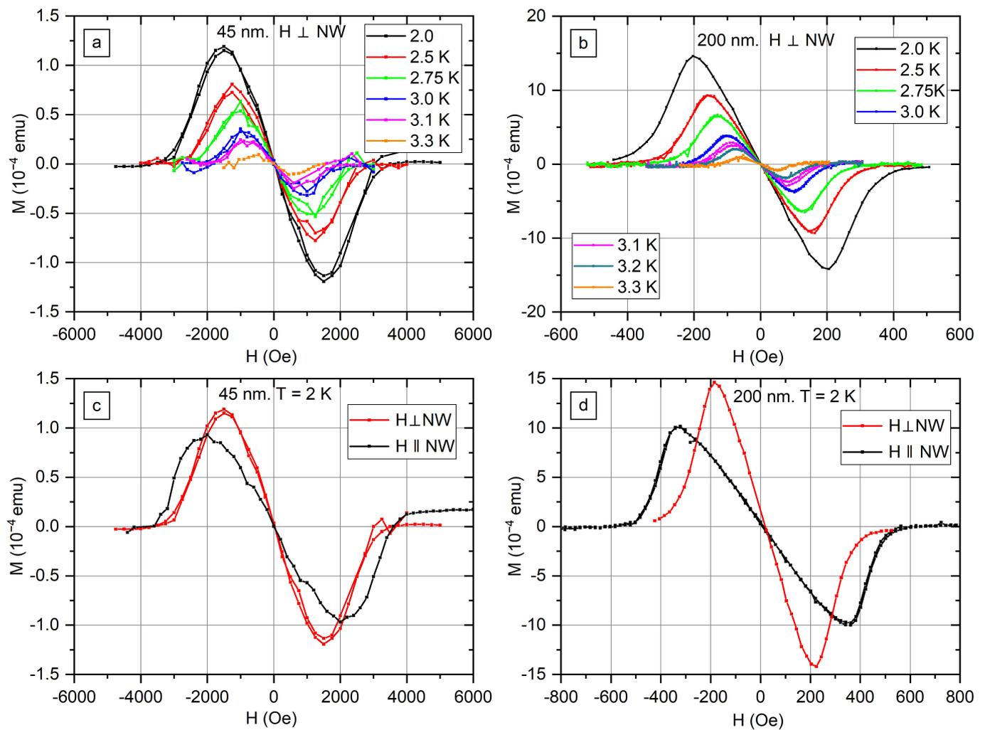
**Figure 5.** The magnetic moment  $M$  as a function of transverse magnetic field  $H$  for In nanowire arrays with nanowire diameters 45 nm (a) and 200 nm (b). The comparison of  $M(H)$  curves measured at 2 K temperature for the same sample in transvers and axial fields: s45 (c) and s200 (d).
