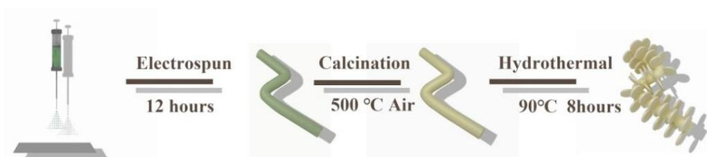
**Scheme 1.** Schematic diagram showing the construction of the NiMoO<sub>4</sub>@Ni(OH)<sub>2</sub> nanofibers.
