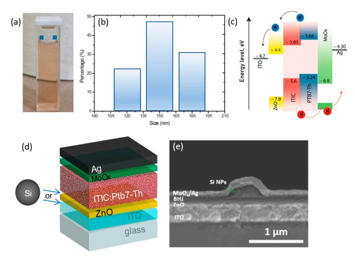
**Figure 1.** (a) Photo of a colloidal solution of Si NPs in isopropanol. (b) Size distribution of Si NPs in the solution. (c) Energy band diagram of the device. (d) Schematic illustration of the architecture of the studied organic solar cells. Arrows indicate the two positions of Si NPs deposition. (e) Cross-sectional SEM image of the obtained device with a single Si NP covered by BHJ/MoO<sub>x</sub>/Ag layers.
