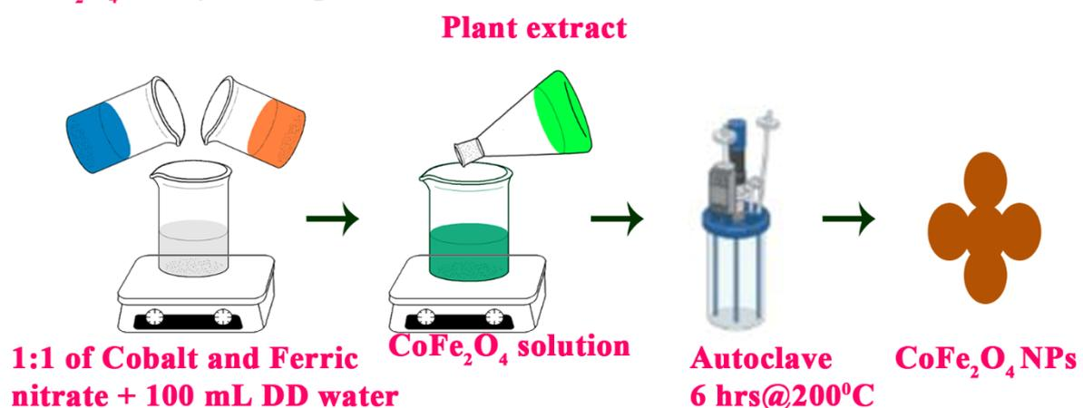
**Scheme 1.** Synthesis protocol of CoFe<sub>2</sub>O<sub>4</sub> NPs.
